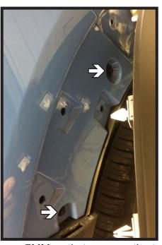
9. Using a 7MM socket, remove the two (2) bolts. Do this on both sides of the vehicle.
