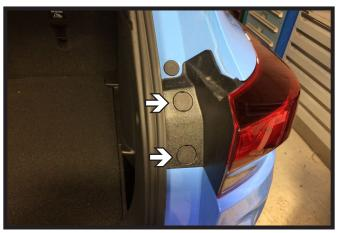
1. Remove the two (2) plastic caps next to the tail light. Do this on both sides of the vehicle.
