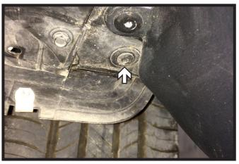
13. Using a T15 Torx, remove the one (1) bolt from behind the tire. Do this on both sides of the vehicle.
