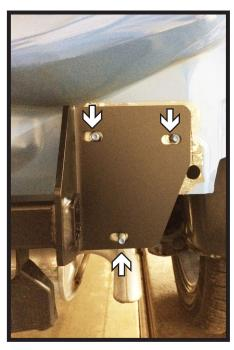
19. Slide the receiver onto the vehicle. Apply clear 100% silicone around the three (3) bolt holes of the receiver. Do this on both sides of the vehicle.
