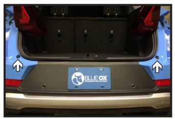
4. Using a T15 Torx, remove the two (2) bolts from below the trail light housing. There is one (1) on each side of the vehicle.
