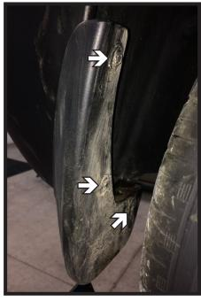
6. Using a T15 Torx, remove the three (3) bolts from the rear mud flap. Do this on both sides of the vehicle.
