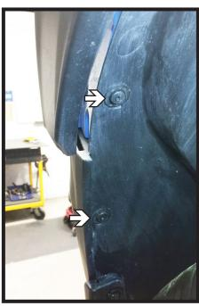
5. Using a T15 Torx, remove the two (2) bolts from the edge of the wheel well. Do this on both sides of the vehicle.
