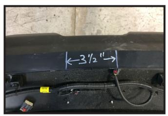
21. Using a reciprocating saw trim the rear fascia to allow clearance for the receiver hitch. Approximately 3-1/2" wide by 2" deep.
