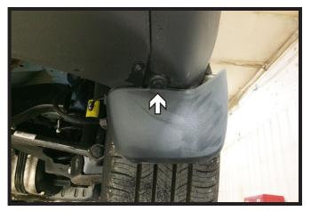
11. Using a T15 Torx, loosen the one (1) bolt behind the tire and rotate outward. Do this on both sides of the vehicle.
