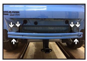
20. Place the rear bumper onto the vehicle. Reinstall the six (6) existing nuts and tighten.
