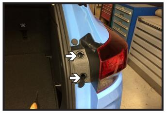
2. Using a T15 Torx, remove the two (2) bolts next to the tail light. Do this on both sides of the vehicle.
