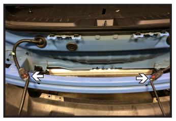
14. As the rear fascia is removed, unplug the two (2) electrical connections. There is one (1) on each side of the vehicle. Remove the fascia and set aside to be reinstalled later.
