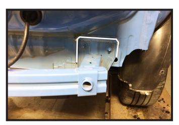
15. Using a utility knife or razor blade, cut around the bumper where it attaches to the frame.
