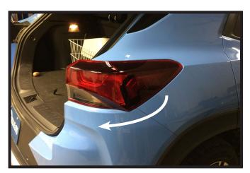
Push tail light toward the rear, remove and let hang. Do this on both sides of the vehicle.
