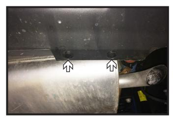
10. Remove the two (2) push pins from the underside of the vehicle. Do this on both sides of the vehicle.
