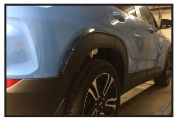
8. Pull back the rear wheel well trim past the fascia joint. Prop trim away from the vehicle using a soft cloth. Do this on both sides of the vehicle.
