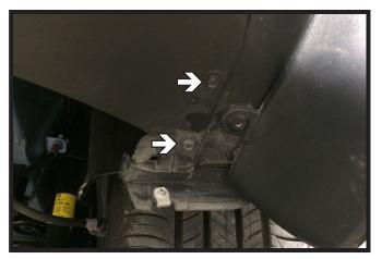
12. Using a 7MM socket, remove the two (2) bolts from behind the tire. Do this on both sides of the vehicle.
