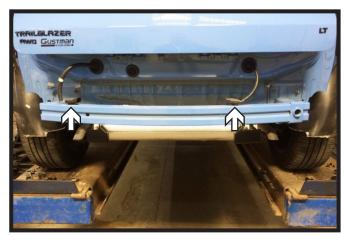
16. Unclip the wire loom from the bumper on each side of the vehicle.
