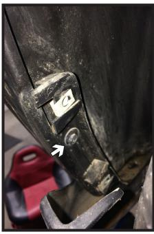
7. Using a 7MM socket, remove the one (1) bolt underneath the mud flap. Do this on both sides of the vehicle.
