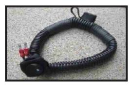
BEFORE YOU BEGIN: Consult the owner's manual for the towed vehicle to determine which fuse must be removed from the "towed" vehicle. Confirm that the pins on the Fuse ByPass Switch wires match the pin sizes on the fuse you removed. You must have the correct fuse wire ends for your fuse box. If your vehicle is equipped with a ATM Micro Mini fuse, a ATM Mini fuse of the same rating as the OEM will need to be installed into the ATM Mini Fuse Bypass Switch holder.
