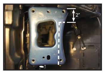
10. Using a reciprocating saw, trim the outer flange of the frame down 2" and back to the face of the frame. Do this on both sides of the vehicle.
