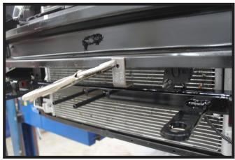
17. **Optional Breakaway:** Position the bracket in the desired location along the bottom lip of the bumper. Clamp and drill a 5/16" hole thru the bumper. Install the bracket to the vehicle with the supplied 1/4" hardware.
