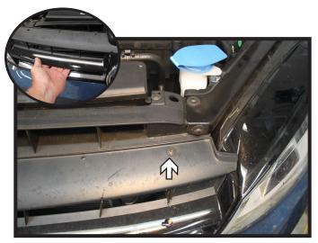
Using a T25 Torx, remove the two (2) screws from the top edge of the grille. There is one (1) on each side. Unsnap the grille from the vehicle and set aside.
