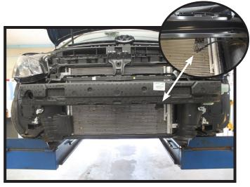
Remove the styrofoam support from the face of the bumper.
