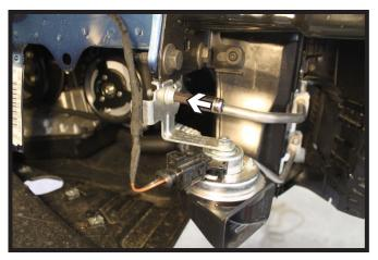
6. Using a 5/16" Allen socket or wrench, remove the screw from the horn bracket and set the horn assembly aside. Do this on both sides of the vehicle.
