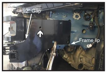
13. Position the baseplate on the vehicle so there is an approximate 1/2" gap between the baseplate and back of the bumper with the baseplate sitting on the lip of the frame. Level and clamp the baseplate.
