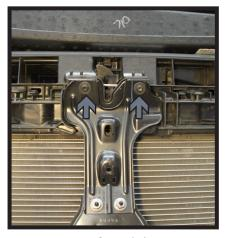
7. Using a 16MM socket, remove the eight (8) bolts from the bumper. There are four (4) on each side, two (2 on top & two (2) on bottom (white).
