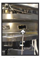
Using a 1-1/4" hole saw, drill an access hole on the underside of the bumper on the passenger side only (left).
