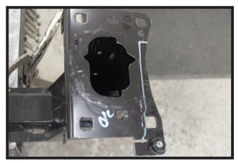
11. Temporarily reinstall the bumper, mark the backside of the flanges to trim to match the frame. Do this on both sides of the vehicle. Remove the bumper and trim the flanges of the bumper. Reinstall the bumper to the vehicle.
