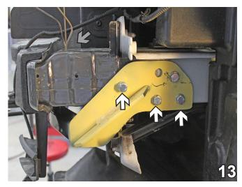
13. Use the 13/32" drill bit and drill out the remaining three (3) holes on each side. Secure each hole with a 3/8"-16 x 1-1/4" hex bolt (white arrows) with a 3/8" lock washer and a 1/4"-20 x 1" x 1" nut plate (gray arrow).
