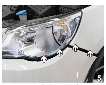
To remove the fascia, carefully lift up and out from the vehicle on the edge near the driver's side front wheel. Do this on both sides. Set the fascia aside to be reinstalled later.
