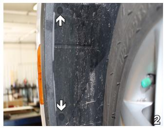
In front of the driver's side front tire, use a T30 Torx and remove two (2) bolts from the wheel well. Do this on both sides of the car. Set bolts aside to be reinstalled later.
