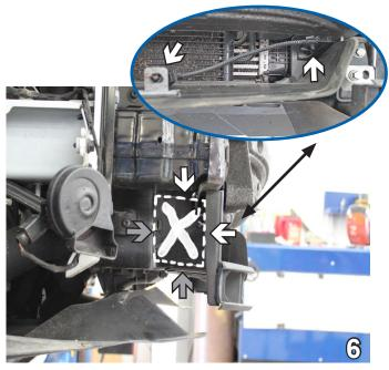
6. Using a utility knife, cut a square from the black plastic radiator cover. Trace the bottom edge and the back edge of the bumper for two (2) sides of the cut (white arrows), and to the back and bottom of the plastic for the other two (2) sides (gray arrows). Do this on both sides of the vehicle. On the driver's side, unplug electrical connection.
