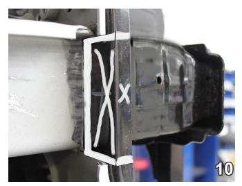
10. Reinstall the front bumper using the existing hardware. Then, use the cut you just made as a template and outline the cut on the back of the front bumper. Use a reciprocating saw and cut this outline out on both sides of the bumper. Reinstall bumper. The radiator cross member will need to be lifted slightly to align holes for bumper reinstallation
