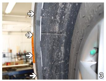
Remove the wheel well trim from the driver's side front wheel. To do this, pinch the trim clips from the inside of the wheel well, after pulling back the wheel well. Do this on both sides. Set all parts aside to be reinstalled later.
