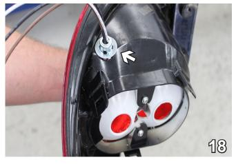
18. Use a 1/2" drill bit, and drill a hole in the back of the tail light. Put the wires through the holes and silicone around it. Reinstall the taillight. Do this on both sides.
