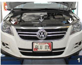
Using a T30 Torx, remove the a bolt from each side of the top of the fascia, near each headlight (white arrows). Use a T25 Torx to remove the bolt from the top of the center of the fascia (gray arrow). Set bolts aside to be reinstalled later.
