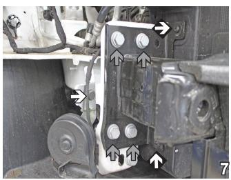
7. Remove the horn brackets using a 13MM socket (white arrows). Then to remove the front bumper, use a 15MM socket and remove the four (4) mounting bolts from each side (gray arrows). Then use a T30 Torx, and remove the last bolt holding the bumper on. Do this on both sides of the vehicle. Set all bolts aside to be reinstalled later.
