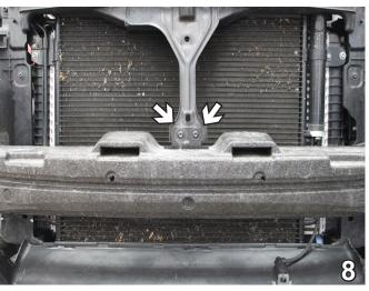
8. Use a T30 Torx to remove the two (2) bolts from the middle of the bumper. Remove the bumper and set bolts and bumper aside to be reinstalled later.
