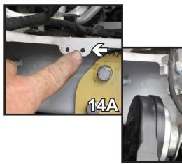
14. On the driver's side, reattach the horn with the existing hardware. On the passenger's side, use a 1/4" dril bit and drill through one (1) of the existing holes on the frame webbing (14A). Secure the passenger's side horn with a 1/4"-20 x 3/4" hex bolt with a 1/4" lock washer a 1/4" hex nut (14B). Tighten with Loctite Red.
