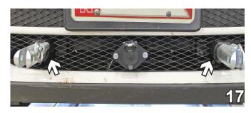
17. Align the fascia to its original position. Trim the grill with a utility knife to allow access to the removable tabs on both sides.
