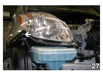
27. Reinstall the headlight. Reconnect all electrical connections and clamps.
