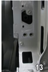
13. Measure up 5/8" from the bottom and across on the lower frame support webbing. Use a reciprocating saw to cut out the notch. Do this on both sides.
