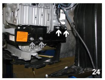
24. Loosen the front two bolts (gray arrows). Insert in the back 3/8"-16 x 1-1/2" bolts, the spacer plates, 3/8" lock washers and 3/8" hex nuts. Loctite Red all bolts and tighten. Then install 3/8" lock washers onto the front two (2) 3/8"-16 x 1" bolts (gray arrows) and 3/8" hex nuts, Loctite Red all bolts and tighten. Do this on both sides.
