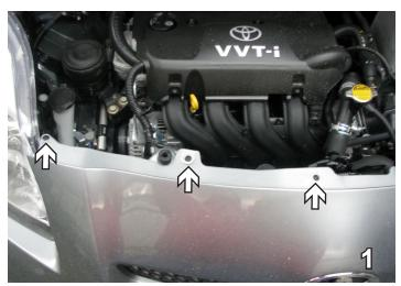
Push in center to remove plastic push pins from top edge of fascia. Set push pins aside to be reinstalled later.
