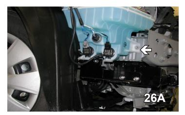
26. **2007-11 Models (28A):** On the passenger side, reinstall the washer reservoir. Reconnect the electrical connections and the hoses.
