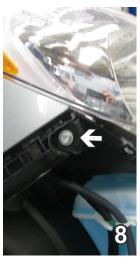
8. On the passenger side, use a 10MM socket to remove the two (2) top screws and one (1) lower screw from headlight. Unhook wiring and set headlight and bolts aside for later reinstallation.
