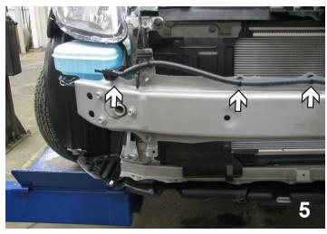
5. **2007-2011 Models Only:** On the back side of the bumper, unhook five (5) hose clamps by squeezing together.
