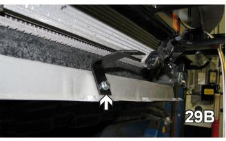
29. Using the hole in the middle of the lower frame. Attach the breakaway bracket with a 6MM-1 x 16MM hex bolt and a 1/4" lock washer inserted into the hole.
