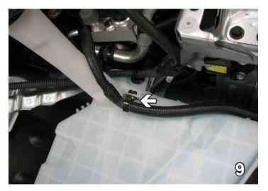
9. On the top of the washer reservoir, squeeze the tab to release the hose.
