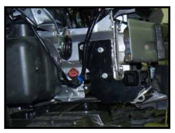
15. Attach the permanent baseplate safety cables to the provided convenience link on the baseplate. Additional options may interfere with suggested mounting; in this case, secure the cables to a solid piece of the frame as described in the instructions included with the permanent baseplate safety cables. Be sure the safety cables do not rub against any hoses or moving parts. Do this on **BOTH** sides of the vehicle.
