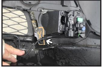
12. On the backside of the fascia, remove the wiring from the clip (white) and trim the inside edge of the fascia as shown. Do this on both sides of the fascia.
