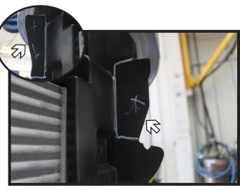
6. Trim the plastic shrouding around the radiator as shown. Do this on both sides of the vehicle.
