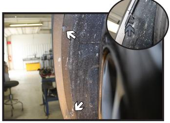
2. In the wheel well, using a Phillips screwdriver, remove the two (2) screws from the outer edge (white). Then using a T27 Torx, remove the screw from the top outer edge (gray).
