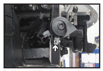
7. Using a 10MM socket, remove the nut from the horn bracket on the passenger side and move the horn aside.
