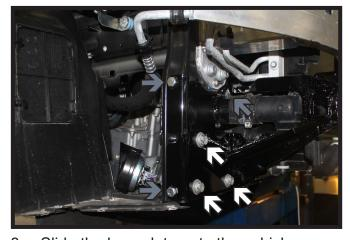
8. Slide the baseplate onto the vehicle. Secure in place with the six (6) existing bolts (white). There are three (3) on each side and fully tighten all hardware. Using a 13/32" drill bit, drill the six (6) holes thru the frame (gray). There are three (3) on each side. Install six (6) 3/8"-13 x 1" bolts into the holes with 3/8" wire nuts on the inside of the frame and fully tighten all hardware.
