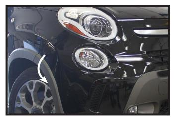
4. Unsnap the fascia from each side. Unplug all electrical connections, then pull the fascia forwards from the vehicle.
