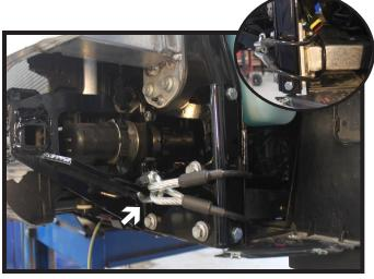
10. Attach the permanent baseplate safety cables to the provided convenience link on the baseplate. The photo above shows the recommended installation of the cables to frame of vehicle. Additional options may interfere with suggested mounting; in this case, secure the cables to a solid piece of the frame as described in the General Information sheet. Be sure the safety cables do not rub against any hoses or moving parts. Do this on **BOTH** sides of the vehicle.
