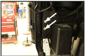
9. Drill two (2) 3/8" holes thru the side plate using the spot welds as a guide. Insert two (2) 3/8"-16 x 1" hex head bolts and 3/8"-16 hex nuts. Do this on both sides on the vehicle.
