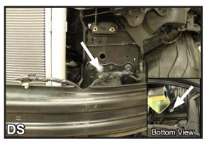
11. For additional support when reinstalling the front bumper you will need to drill two (2) 3/8" holes into the bumper mounting plate. Once the bumper is reinstalled securely, reattach the temperature sensor.
