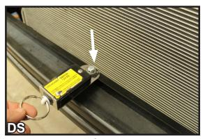
12. To install the breakaway switch measure 15-1/2" from the inside edge of the bracket. Drill a 1/4" hole.
