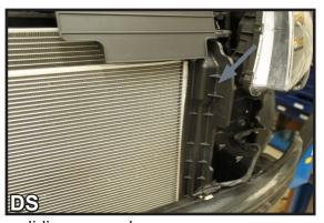
5. Remove the plastic brackets along side the radiator by sliding upward.
