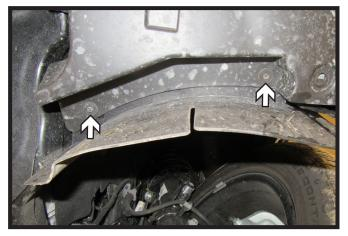
Using a 5.5MM socket, remove the two (2) bolts from in front of the tire on the underside of the vehicle. Do this on both sides of the vehicle. Remove belly pan and set aside to be reinstalled later.
