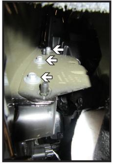
4. Pull back the wheel well liner. Using an 8MM socket, remove the three (3) bolts from the wheel well joint. Do this on both sides of the vehicle.
