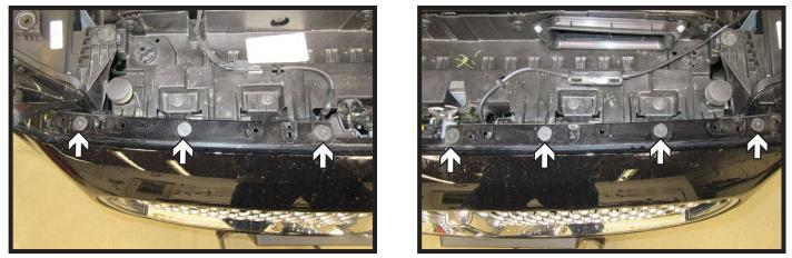
2. Using a T20 Torx, remove the seven (7) screws from the top of the fascia. There are four (4) on the driver side and three (3) on the passenger side.
