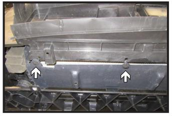
Remove the four (4) push pins from along the underside of the shutter housing. There are two (2) on each side. Remove plastic piece, it will not be reinstalled later.
