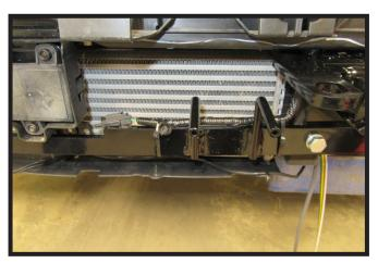
23. Using the provided zip ties, reattach the temperature sensor loom to the top of the baseplate cross member as shown.
