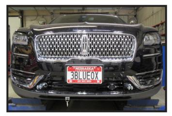
26. Hold the fascia as close to its original position, mark and trim the fascia around the convenience links and attachment tabs. Reinstall the fascia, belly pan, and fascia cover.
