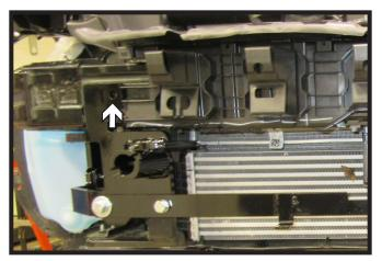
21. Using a 1/2" drill bit, drill one (1) hole as indicated on both sides of the vehicle.
