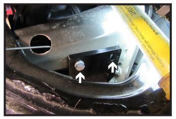
Install the baseplate onto the frame with the provided 3/8" hardware, making sure to not yet fully tighten the hardware. Do this on both sides of the vehicle.
