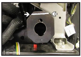
Using a reciprocating saw, trim the marked area on the front of the lower support. Do this on both sides of the vehicle.
