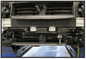
20. Attach the permanent baseplate safety cables to the provided convenience link on the baseplate. The photo above shows the recommended installation of the cables to frame of vehicle. Additional options may interfere with suggested mounting; in this case, secure the cables to a solid piece of the frame as described in the General Information sheet. Be sure the safety cables do not rub against any hoses of moving parts. Do this on **BOTH** sides of the vehicle.
