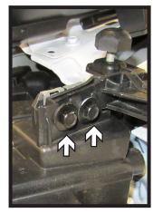
6. Using a T25 Torx, remove the one (1) screw from the plastic headlight cover (white, left). Remove the two (2) push pins (black). Pull the plastic cover up. Using a 10MM socket, remove the two (2) exposed bolts (white, right). Do this for both sides of the vehicle.
