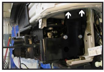
13. Install the baseplate onto the frame with the 3/8" hardware. Level the baseplate prior to fully tightening the bolts. Do this on both sides of the vehicle. (Upper bolts not pictured)
