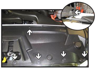
Remove the ten (10) push pins from the fascia cover. There are five (5) on each side. On the driver side, remove one (1) push pin and unhook the cover. Set the cover aside.
