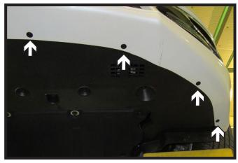
4. Using a 7MM socket, remove the eight(8) bolts from the underside of the fascia.There are four (4) bolts on each side.
