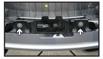
Using a 8MM socket, remove the two (2) bolts from the top side of the bumper. Unhook any electrical connections and pull the bumper from the vehicle.
