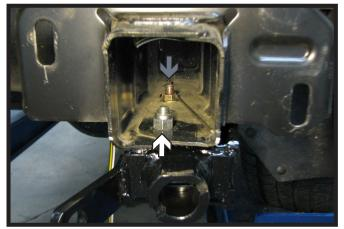
The front bolt (white) uses a 1/2"-13 nylon hex nut. The back bolt (gray) uses a 1/2"-13 whiz nut plate. Tighten down while pushing the plate toward the frame. Do this to both sides.
