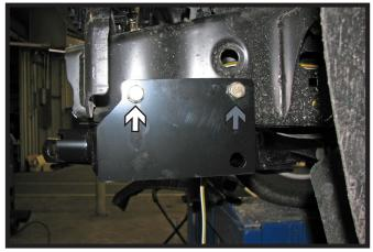
With the baseplate as a template, use a 17/32" drill bit to drill the two (2) holes on the sides of the baseplate. Insert a 1/2"-13 x 1-3/4" hex bolt, 1/2" lock washer and 1/2"-13 nylon hex nut into the front hole (white). Then insert a 1/2"-13 x 1-3/4" bolt, 1/2" lock washer and 1/2"-13 whiz nut plate into the back hole (gray).
