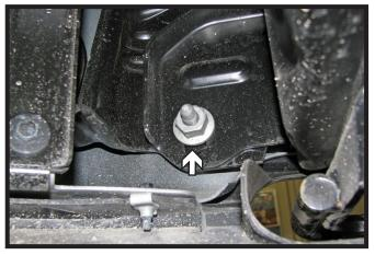
2. From the underside of the bumper, using a 21MM socket, remove the bolt from the outer side of the frame. Do this on both sides of the vehicle.
