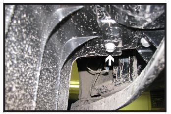
4. **2010-11 Models:** Using a 13MM socket, remove the lower air dam from the vehicle. The air dam will not be reinstalled.
