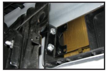
Install the electrical bracket on either side of the vehicle depending on the location of the plug in of the coach. Hold up the bracket and mark on the back side. Attach with 1/4"-20 x 3/4" hex bolts, 1/4" lock washers, 1/4" flat washers and 1/4"-20 whiz nuts.
