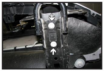
5. Remove the tow hook from both sides by removing the two bolts using a 15MM socket. Set tow hooks and bolts aside, they will not be reinstalled.
