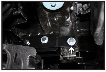
Using a 17/32" drill bit, drill the rear side plate hole thru the tow hook bracket. Install a 1/2"-13 x 1-1/2" bolt with 1/2" lock and flat washers into the hole with 1/2" nut wires on the inside of the bracket and tighten. Do this on both sides of the vehicle.
