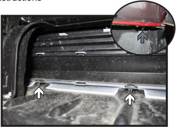
2. Remove the seven (7) push pins (white) and the two (2) plastic rivets (gray) from the inside edge of the spoiler where it meets the bumper. Set the spoiler aside.
