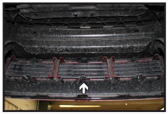
3. From inside the bumper, unclip the front cover from the bumper and set the cover aside.
