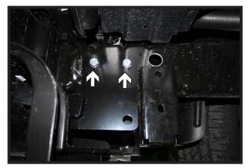
Using a 17/32" drill bit, drill the upper two (2) holes of the baseplate thru the frame. Install 1/2"-13 x 1-1/2" bolts with 1/2" lock washers into the holes with 1/2" nut wires on the inside of the frame and tighten. Do this on both sides of the vehicle.
