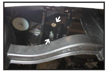
Using a 17/32" drill bit, drill the bottom two (2) holes of the baseplate thru the frame. Install 1/2"-13 x 1-1/2" bolts with 1/2" lock washers into the holes with 1/2" nut wires on the inside of the frame and tighten. Remove the clamps. Do this on both sides of the vehicle.
