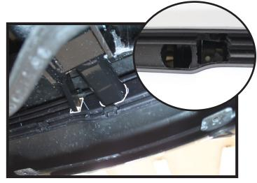
5. Temporarily reinstall the front cover. Hold the baseplate up as close to its installed position. Mark the backside of the front cover. Remove and trim the cover to allow the baseplate to pass thru. Do this on both sides of the vehicle.
