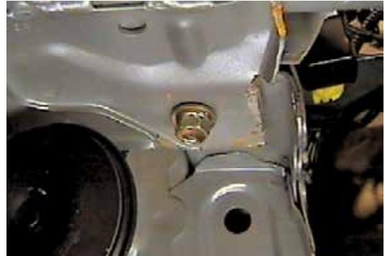
8. Remove one metric bolt from the bottom side of metal bumper using the 12MM socket, pull forward and set aside.
