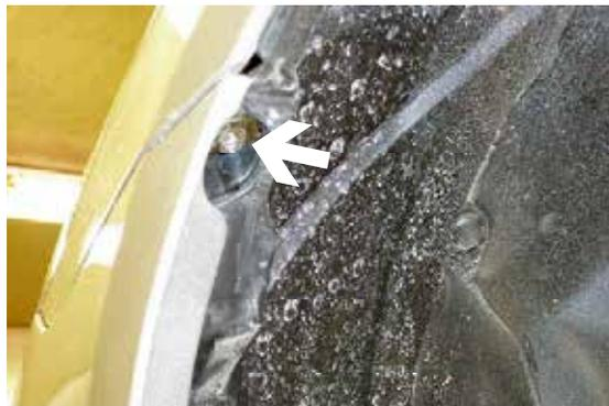
3. Just forward of front tire is one metric bolt to remove, using the 8MM socket, both sides, pull fascia down on the ends and forward, set aside.
