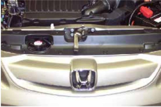
1. Remove the eight push pins from black plastic cover on top side of fascia, lift cover and set aside.
