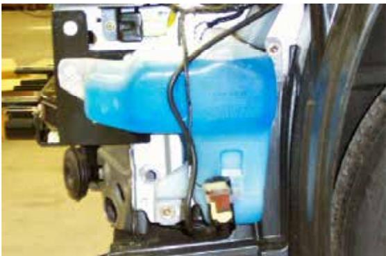
16. Reinstall washer reservoir on the driver's side with existing back bolts and replace existing front bolt with the 6MM-1 x 45MM hex bolt, 1/4" flat and lock washer (Do not over tighten). **2005 MODEL:** Use the 6MM-1 x 30MM hex bolt.
