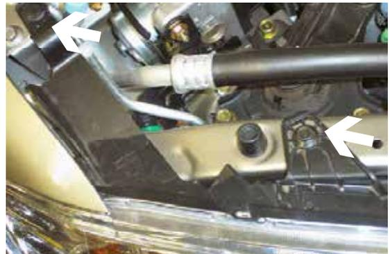
4. Using the 10MM socket, remove one metric bolt and one push pin from the top side of headlight assembly, both sides.
