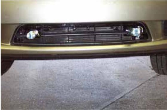
17. Hold fascia to its original position and trim horizontal rib to allow attachment receivers to come through. **OPTIONAL METHOD:** Remove lower black plastic from the back side of fascia's opening.
