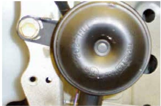
10. Using the 12MM socket, remove the metric bolt from horn bracket on driver's side.
