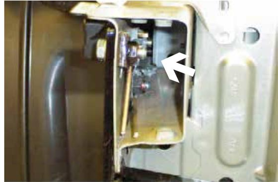
14. Using the flat chisel, remove the square nut attached to the inside of the frame that aligns with existing hole in frame on the passenger's side (see white arrow in step 15).
