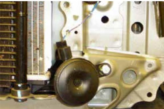
11. Relocate horn bracket to existing hole just below original location using the 5/16-18 x 3/4" hex bolt, lock washer and whiz nut.
