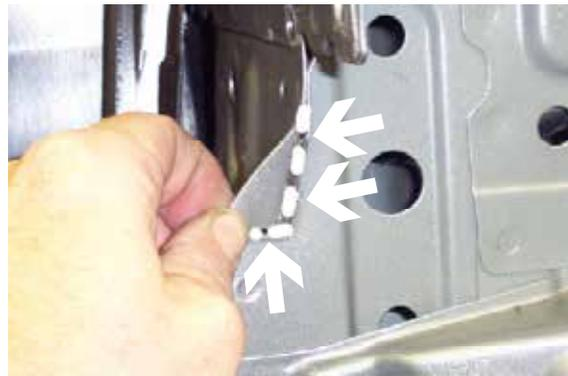
12. Cut and remove forward webbing on lower frame with the hack saw or reciprocating saw, both sides.
