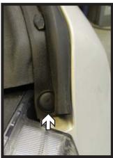
1. Remove the four (4) push pins from the top of the fascia cover and the two (2) push pins from the inside point near the headlights. Remove fascia cover and set aside.
