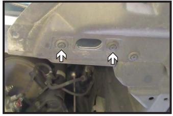
7. On the passenger side, remove two (2) push pins under the windshield wiper fluid reservoir with a Phillips screwdriver.
