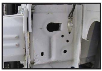
12. On the side of the frame rail, using a reciprocating saw, make two horizontal cuts (between 1" - 1 1/2" long) as shown on the existing hole. Trim additional metal from the area. Do this on both sides of the vehicle.
