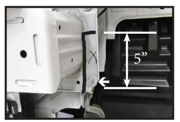
11. Using a 12MM socket, remove outer bottom bolt on bumper horn. With a reciprocating saw, trim the bumper horn five inches up from the bottom, flush with the face of the frame. Do this on both sides of the vehicle.
