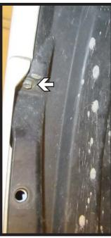
3. In front of the tire, remove three push pins (right). Also in front of the tire, using an 8MM socket, remove the single bolt from the upper wheel well (left). Do this on the both sides.
