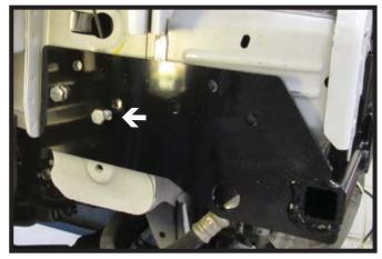
13. Slide the baseplate Into position and insure it is level and aligned with existing holes, before clamping to the frame rail on both sides with large vise grips. On the driver's side, insert 3/8-16 x 1 1/2" hex bolt with 3/8" lock washer into existing hole with the 3/8" nut plate on the inside of the frame. Do this on both sides of the vehicle. Fully tighten all hardware.
