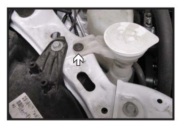
10. Remove the one (1) push pin from the reservoir neck, remove the reservoir and set aside.
