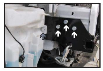
14. On the driver's side, drill five holes with a 3/8" drill bit. Insert 3/8-16 x 1 1/2" hex bolt with 3/8" lock washer into drilled holes, with the 3/8" nut plate on the inside of the frame. Complete these steps on the passenger side. Fully tighten all hardware.
