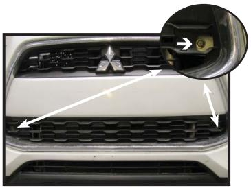
4. Using a 10MM socket, remove the two (2) bolts from the front of the fascia.
