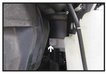
9. To remove the washer reservoir, you must first unplug the electrical connections, disconnect and plug the fluid lines (pictured with gray arrows). Using a 12MM socket, remove two (2) bolts from the front of the reservoir, and one (1) from the back (right).
