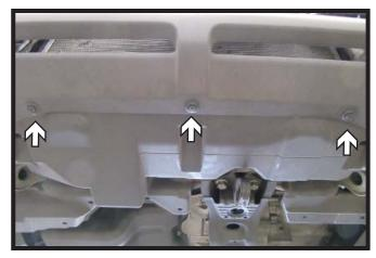
5. Using a Phillips screwdriver, underneath the fascia, remove the eleven (11) push pins. There will be four (4) on each side and three (3) in the center.
