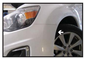
6. Pull the corners of the fascia away from the vehicle disconnecting any electrical connections and set the fascia aside.
