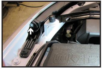
3. Using a 10MM socket, remove the one (1) bolt from the fascia joint. Do this on both sides of the vehicle.
