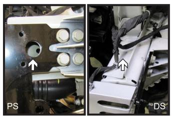
17. Using a 1-1/4" hole saw, drill access hole using the bracket template on the passenger side and drill hole in indicated area on the driver side of the vehicle.
