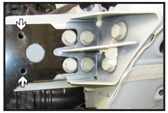
18. Make sure that the side bracket is level. Then using a 3/8" drill bit, drill out the two (2) middle holes. Do this on both sides of the vehicle.
