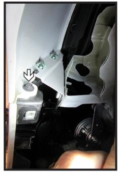
5. Pull back the wheel well liner. Using a 7MM socket, remove the one (1) bolt from the fascia joint. Do this on both sides of the vehicle.
