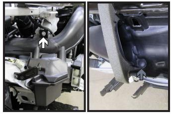
8. Using a 10MM socket, remove the one (1) bolt (white) and one (1) push pin (gray) from the air dam on the passenger side of the vehicle. Remove air dam and set aside to be reinstalled later.
