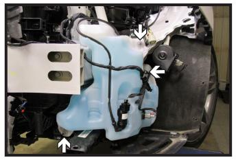
Using a 10MM socket, remove the three (3) nuts from the windshield washer fluid reservoir on the driver side of the vehicle. Remove reservoir and set aside to be reinstalled later.
