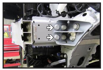
12. Using an 18MM socket, remove the front two (2) bolts on the side of the frame. Do this on both sides of the vehicle.
