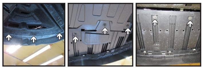
6. Using a 7MM socket, remove the fifteen (15) bolts from the underside of the fascia. There are six (6) on each side and three (3) in the middle.
