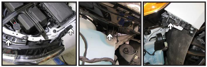
7. Using a 7MM socket, remove the four (4) bolts from the head light. There are two (2) on top, one (1) in front, and one (1) on the side. Remove head light and set aside to be reinstalled later. Do this on both sides of the vehicle.
