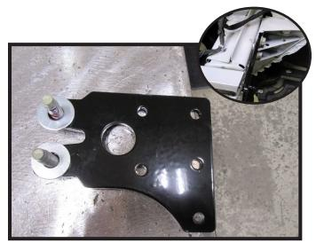
16. Install side plate using the two (2) existing 12MM bolts and provided hardware. Make sure that the flat washers are between the baseplate and the frame and the plate is level (inset). Do this on both sides of the vehicle.
