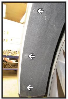
4. Using a T15 Torx, remove the three (3) screws from along the edge of the wheel well. Do this on both sides of the vehicle.
