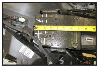
14. Using a reciprocating saw trim 2" inches as shown from each end of the Styrofoam on the back of the fascia.
