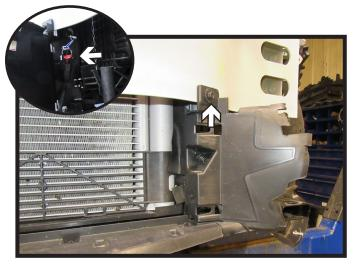
Using a 7MM socket, remove the two
