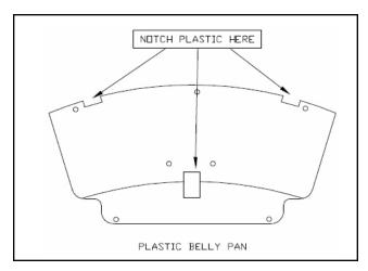
NOTE: Do not bolt the center brace to the frame. It will be easier to fasten the lower plastic belly pan.
