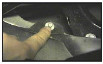
2. Using a 6MM socket, remove the nine (9) screws from air dam and set aside.
