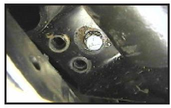
5. Install the baseplate into the tow hook pocket aligning the back hole. Install the 1/2" hardware and fully tighten. Do this on both sides of the vehicle.
