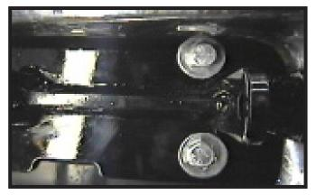
6. Reinstall the four (4) existing bolts back into the bumper openings and fully tighten.
