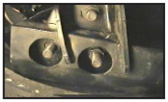
1. Using a 21MM socket, remove the three (3) bolts from the cross member. Do this on both sides of the vehicle and set the cross member aside.
