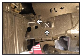
2. Remove the plastic plug from the frame (right). Then trim off the lower part of the plastic shielding for baseplate clearance (left). Do this on both sides of the vehicle.
