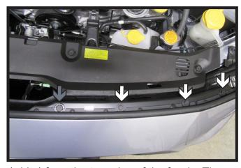
1. Using a 10MM socket, remove the four (4) bolts (white) from the top edge of the fascia. Then remove the two (2) push pins (gray).
