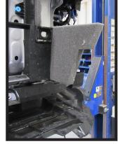
16. Remove the foam pieces from each side on the front of the vehicle.
