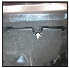
4. Using a Phillips screw driver remove the three (3) plastic screws from the underside of the fascia.
