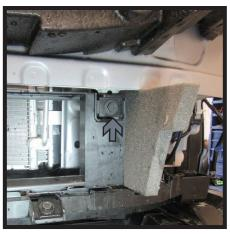
6. Using a 12MM socket, remove the four (4) bolts (white) from the bumper as indicated. Then using a 10MM socket remove the one (1) bolt (gray). Do this on both sides of the vehicle. Remove bumper, it will not be reinstalled later.
