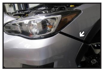
5. Grasp the fascia near the headlight and pull upward and outward to remove. Set aside to be reinstalled later.
