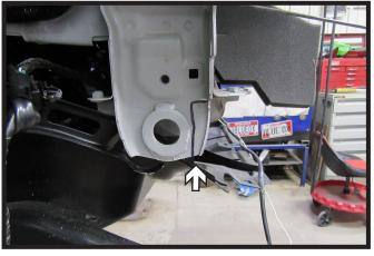
13. After the two (2) previous flanges are trimmed off. Mark and trim the frame flange as shown. Do this on both sides of the vehicle.
