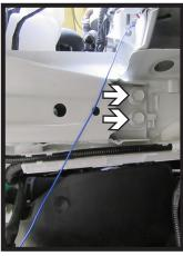
9. On the driver side of the vehicle, using a 14MM socket, remove the four (4) bolts from the frame extension. There are two (2) in the back and two (2) in front. Set the extension aside to be reinstalled later.
