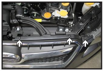
1. Remove the six (6) push pins from the top edge of the fascia. There are three (3) on each side.
