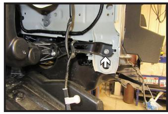
8. Using a 12MM socket, remove the one (1) bolt attaching the bracket on the passenger side of the vehicle. Unclip the wire loom from the frame on both sides of the vehicle.
