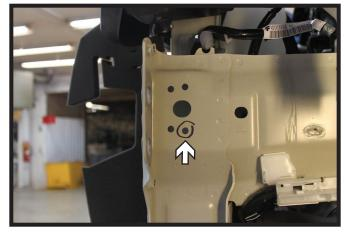
15. Using a 3/8" drill bit, ream out the back bottom factory hole on both sides of the vehicle.
