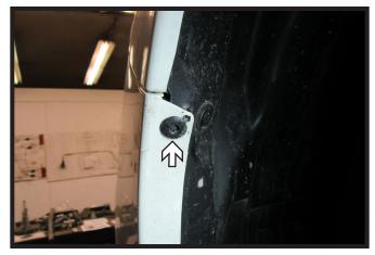
2. Release the push pin from the top edge of the fascia/wheel well joint by pushing in on the center section. Do this on both sides of the vehicle.
