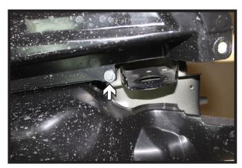
6. Using a 10MM socket, remove the bolt on the underside of the outer plastic shielding, letting the shield hang loose. Do this on both sides of the vehicle.
