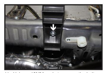
11. Using a 10MM socket, remove the bolt from the belly pan bracket and set aside. Do this on both sides of the vehicle.
