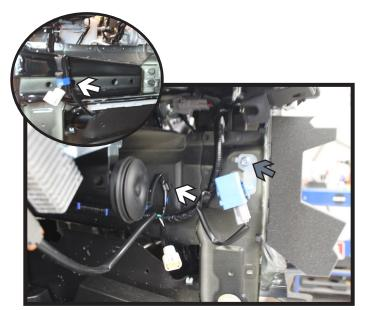
8. On the passenger side, using a 10MM socket, remove the box from the frame and set aside (gray). Also remove the wire loom from the frame (white). On the driver side, unsnap the wire loom from the frame brace (inset).
