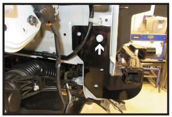
16. Position the baseplate onto the frame. Install a 3/8"-16 x 1-1/2" bolt with 3/8" lock washer into the pre-drilled hole and a 3/8" nut plate on the inside of the frame. Do this on both sides of the vehicle.
