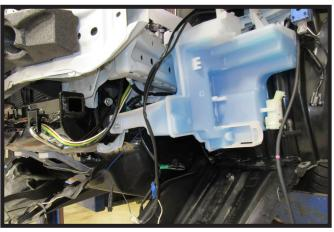
20. Reinstall the windshield washer fluid reservoir attaching it to the frame and baseplate as shown using the existing and provided hardware.
