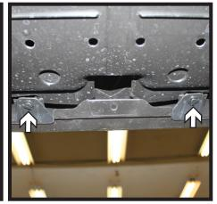
3. Remove the eight (8) push pins from the underside of the fascia. There are three (3) in each corner and two (2) in the middle.
