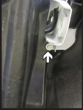
5. Using a 10MM socket, remove the two (2) bolts on the underside of the outer plastic shielding, letting the shield hang loose. Do this on both sides of the vehicle.
