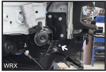
18. **XV/Impreza:** On the passenger side, reattached the box to the frame just below the horn using the supplied self tapping screw.
