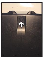
3. Remove the nine (9) push pins from the underside of the fascia. There are four (4) on each side and one (1) in the middle. Unsnap the corners of the fascia from the fender. Remove the fascia from the vehicle, disconnecting any electrical connections and set the fascia aside.
