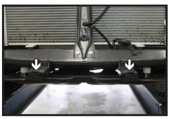
9. Unsnap the belly pan from the two plastic pieces on the front of the vehicle.
