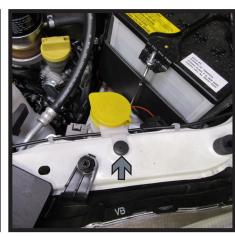
6. Using a 10MM socket, remove the three (3) bolts (white) from the washer reservoir. There is one (1) in front, one (1) at the top and one (1) behind the wheel well liner. Remove the Phillips push pin (gray) from the reservoir neck. Disconnect and plug all lines. Set the reservoir aside to be reinstalled later.
