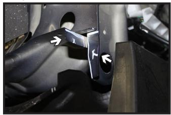
12. Using a reciprocating saw, trim the frame flanges as shown. Do this on both sides of the vehicle.
