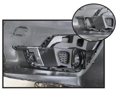
22. **Impreza:** Trim the indicated area on the back of the fascia to allow baseplate clearance. See completed trimmed area in inset.
