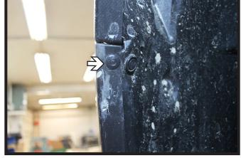
Release the pin from the top edge of the fascia/wheel well joint by pushing in on the center section. Do this on both sides of the vehicle.
