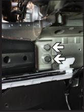
9. On the driver side, using a 14MM socket, remove the four (4) bolts from the frame brace. There are two (2) in the back and two (2) in front. Set the extension aside to be reinstalled later.
