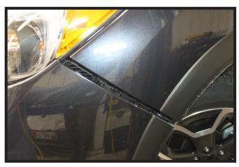
4. Unsnap the corners of the fascia from the fender. Remove the fascia from the vehicle, disconnecting any electrical connections and set the fascia aside.
