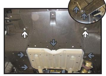
Using a 12MM socket, remove the two (2) bolts (white) and four (4) push pins (gray) from the belly pan. Let belly pan hang out of the way.
