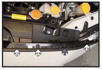
1. Using a 10MM socket, remove the six (6) bolts (white) and three (3) push pins (gray) from the top of the fascia cover. Remove fascia cover and set aside to be reinstalled later.
