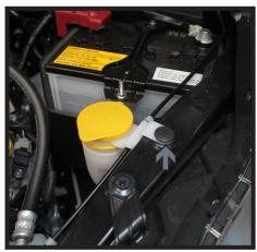
7. Using a 10MM socket, remove the three (3) bolts (white) from the washer reservoir. There is one (1) in front, one (1) at the top and one (1) behind the wheel well liner. Remove the Phillips push pin (gray) from the reservoir neck. Disconnect and plug all lines. Set the reservoir aside to be reinstalled later.
