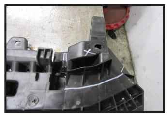
22. **WRX:** Trim the lower shield as needed to clear the baseplate/safety cables. Reinstall lower shield.
