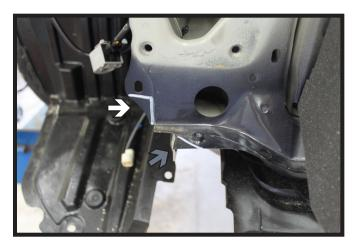
14. Using a reciprocating saw, trim off the corner or bend down (gray). Do this on both sides of the vehicle.
