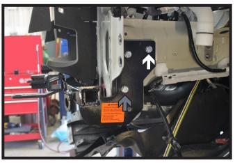
17. Using a 3/8" drill bit, drill the remaining two (2) holes thru the frame. Install 3/8"-16 x 1-1/2" bolt with 3/8" lock washer into the top hole (white) and a 3/8"-16 x 2" bolt with 3/8" lock washer into the bottom hole (gray). Using 3/8" nut plates on the inside of the frame. On the lower hole use the provided spacer tube in between the baseplate and frame. Do this on both sides of the vehicle. Fully tighten all hardware.
