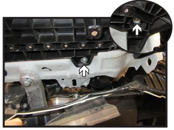
11. Using a 10MM socket, remove the five (5) bolts from the underside of the plastic shield. There are three (3) along the center and one (1) in each corner (inset). Remove shield and set aside to be reinstalled later.
