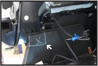
19. Hold the plastic shielding up close to its original position. Mark and trim the shielding around the baseplate. Do this on both sides of the vehicle. Reinstall both sides.
