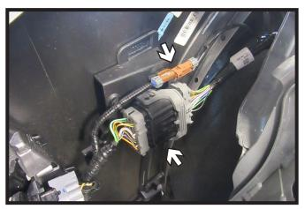
7. Disconnect the two (2) electrical connections on the passenger side of the vehicle.
