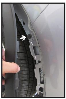
Pull back the wheel well trim and hold in place with a soft cloth. Remove the one
