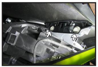
4. Pull back the wheel well trim. Using a 10MM socket, remove the two (2) bolts from the fascia joint. Do this on both sides of the vehicle.
