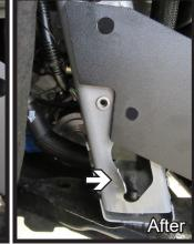
17. Using a pair of large vise grips bend back the frame piece as shown to create and access hole for the baseplate. Do this on both sides of the vehicle.
