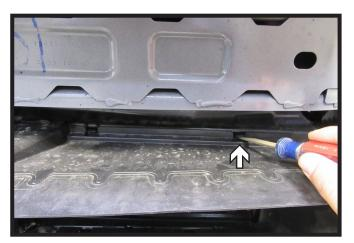
11. Remove the shroud around the lower shutters by removing the two (2) push pins, one (1) on each side of the vehicle. Then using a flat screw driver, remove the eight (8) clips around the edge of the shroud.
