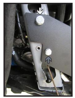
18. Insert nut plate through hole in the frame (left). Insert a 1/2" bolt with lock washer into the top hole (white) and a 3/8" bolt with lock washer into the bottom hole (gray). Do this on both sides of the vehicle.
