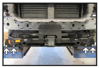
12. Slide the baseplate onto the vehicle and reinstall the four (4) existing 8MM bolts and washers, two (2) on each side. Use level to ensure baseplate is level before tightening bolts.
