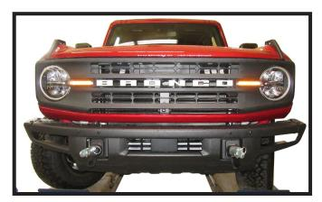
9a. Reinstall belly pan. Hold tow hook cover as close to its original position, mark and trim the covers as needed. Reinstall the covers.
