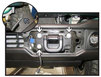
Using a 15MM socket, remove the three
