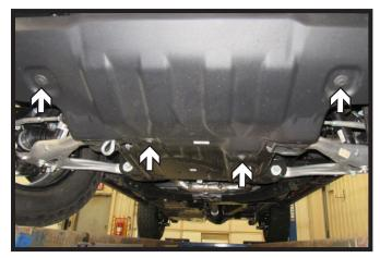
Using a 15MM socket, remove the four
