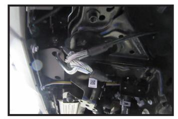
cables to the provided convenience link on the baseplate. The photo above shows the recommended installation of the cables to frame of vehicle. Additional options may interfere with suggested mounting; in this case, secure the cables to a solid piece of the frame as described in the General Information sheet. Be sure the safety cables do not rub against any hoses or moving parts. Do this on **BOTH** sides of the vehicle. Reinstall belly pan.
