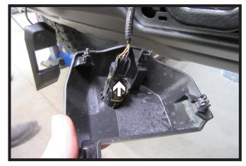
1. Unsnap D-ring cover. Unplug the sensor from the back of the cover. Remove and set cover aside to be reinstalled later. Do this on both sides of the vehicle.
