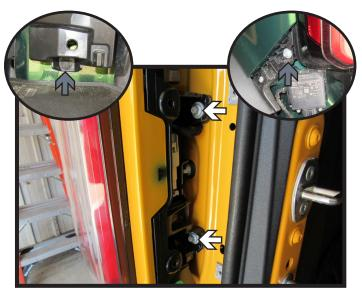
4. Using an 8MM socket, remove the two (2) bolts (white) and using a 10MM socket remove the two (2) bolts (gray, insets) attaching the tail light housing to the frame. Remove the tail light housing and install tail light wiring kit per kit instructions. Do this on both sides of the vehicle.
