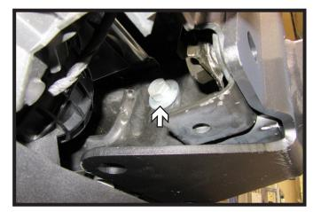
3. Install the two (2) 1/2" bolts with flat washer and lock washer, one (1) on each side of the frame. Do this on both sides of the vehicle.
