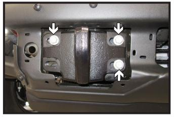
Using a 15MM socket, remove the three
