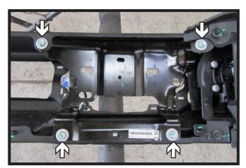
Using a 13MM socket, remove the four
