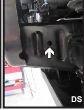
3. Using a 1/2" drill bit, drill out hole on the out side of the frame. Do this on both sides of the vehicle.
