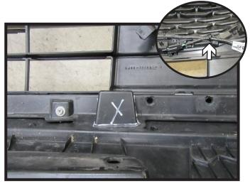
22. Unsnap temperature sensor from the back of the fascia (left). Cut plastic piece from the back of the fascia as shown (right). Zip tie the temperature sensor to the wire loom slightly above previous position (inset).
