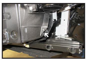
12. On the driver side of the vehicle, notch the plastic piece as shown for baseplate clearance.
