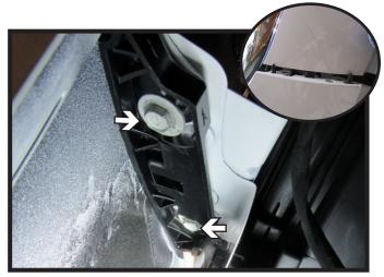
4. Pull back the wheel well liner and remove foam pieces. Using a 10MM socket, remove the two (2) bolts from the underside of the fascia joint. Pull fascia joint apart (inset). Do this on both sides of the vehicle.
