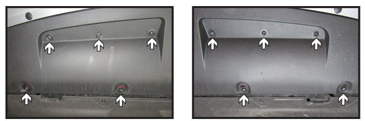
6. Using a T30 Torx, remove the ten (10) bolts, five (5) on each side, from the underside of the fascia.
