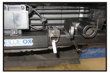
15. **Optional Breakaway:** If installing a breakaway switch, install on baseplate before installing baseplate on vehicle.
