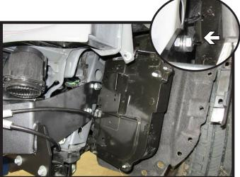
21. Reinstall the black box onto the driver side of the vehicle. Reattach the wire loom to the bottom bolt on the backside. If the box touches the baseplate bolt head, bend back plate slightly to create clearance (inset).
