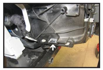
11. On the passenger side of the vehicle, notch the plastic as indicated for baseplate clearance.
