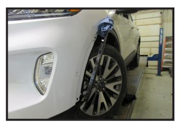
3. Pull back the wheel well trim and prop away from the vehicle using a soft cloth to protect the vehicle. Do this on both sides of the vehicle.
