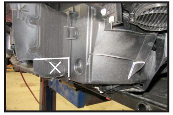
10. Using a utility knife, trim the plastic shroud as shown on both sides of the vehicle.
