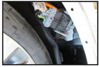
5. On the passenger side of the vehicle, unplug the electrical by pushing down on the center piece while pulling down on the light gray piece.
