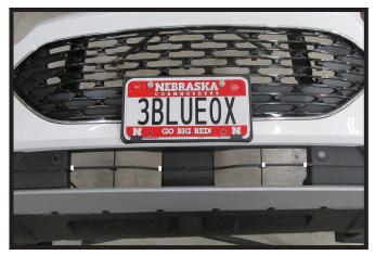
24. Remove the (2) horizontal slats between the white marks as shown to allow room for the removable tabs and convenience links.
