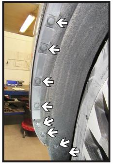
2. Remove the eight (8) push pins from along the edge of the wheel well. Do this on both sides of the vehicle.
