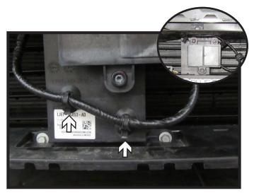
9. Pull out the two (2) plastic pieces holding the wire loom below the Adaptive Cruise Control (ACC). Pull up the shutter housing above the ACC sensor and tuck wire loom between ACC and housing, out of the way of the shutters.
