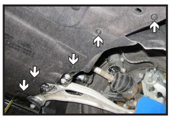
13. Using a 7MM socket, remove the five (5) bolts from belly pan. Do this on boths side of the vehicle. Let belly pan hang loose.
