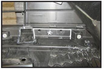
23. On the back of the fascia trim the indicated areas on both sides of the vehicle to allow room for baseplate clearance.
