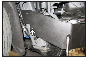
17. Using a 3/8" drill bit, drill out the bottom hole on the side of the frame using the baseplate as a guide. Do this on both sides of the vehicle.
