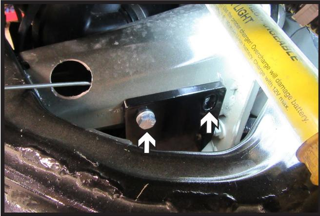
18. Install the baseplate onto the frame with the provided 3/8" hardware, making sure to not yet fully tighten the hardware. Do this on both sides of the vehicle.
