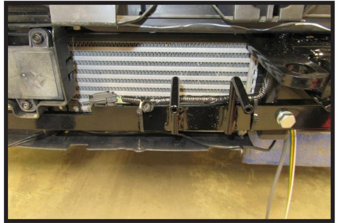
23. Using the provided zip ties, reattach the temperature sensor loom to the top of the baseplate cross member as shown.
