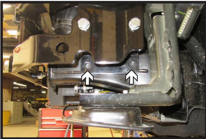
20. Using a 3/8" drill bit, drill out the bottom two (2) holes using the holes on the side plate as a guide. Install the provided 3/8" hardware. Do this on both sides of the vehicle.
