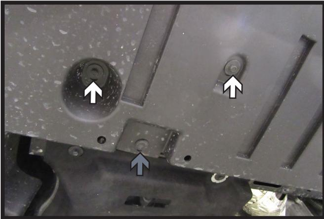
6. Using a 7MM socket, remove the two (2) bolts (white) and one (1) push pin (gray) from the belly pan. Do this on both sides of the vehicle.
