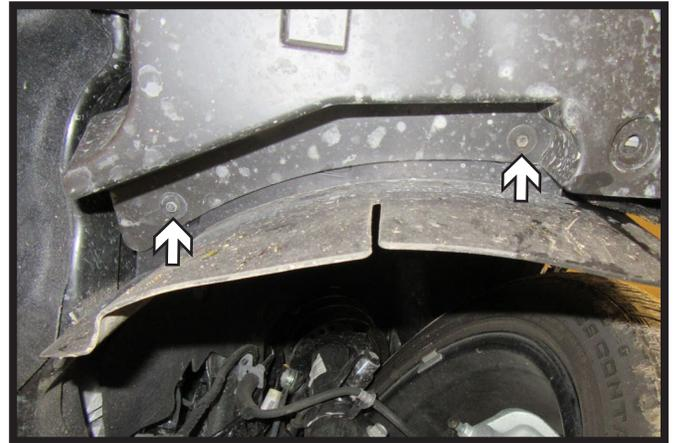
7. Using a 5.5MM socket, remove the two (2) bolts from in front of the tire on the underside of the vehicle. Do this on both sides of the vehicle. Remove belly pan and set aside to be reinstalled later.
