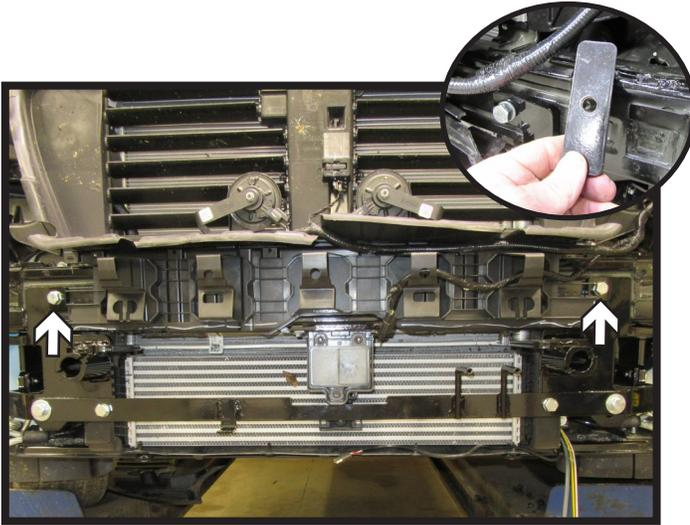
22. Install the 1/2" bolts with lock washer and a nut plate (inset) on the back side. Do this on both sides of the vehicle.
