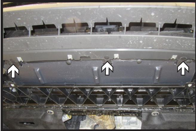
8. Remove the three (3) push pins from the underside of the vehicle. Remove the fascia and set aside to be reinstalled later.
