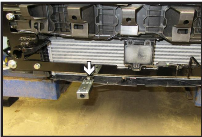
24. **Optional Breakaway:** Using the provided 1/4" hardware, attach the breakaway switch to the bracket on the baseplate as shown.
