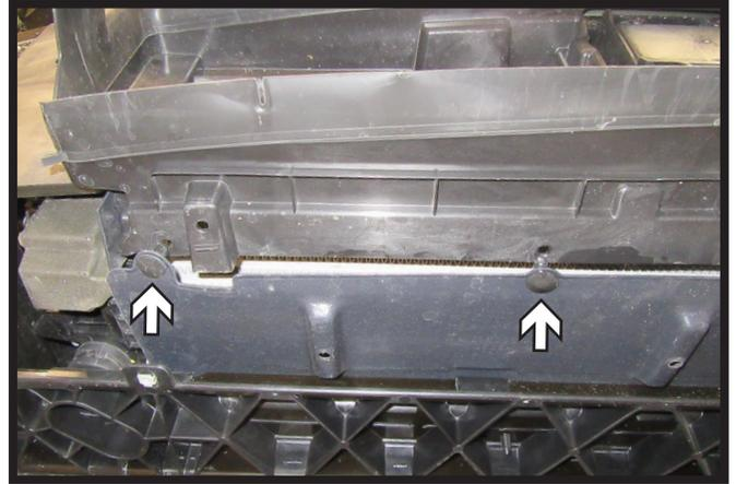
11. Remove the four (4) push pins from along the underside of the shutter housing. There are two (2) on each side. Remove plastic piece, it will not be reinstalled later.
