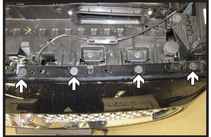
2. Using a T20 Torx, remove the seven (7) screws from the top of the fascia. There are four (4) on the driver side and three (3) on the passenger side.
