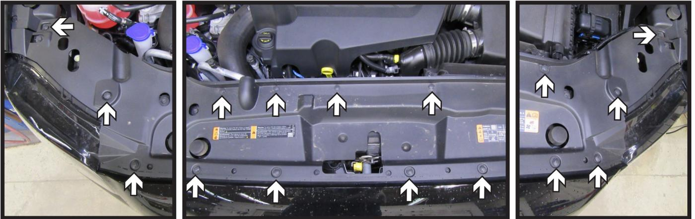
1. Remove the sixteen (16) push pins from the fascia cover. Set cover aside to be reinstalled later.
