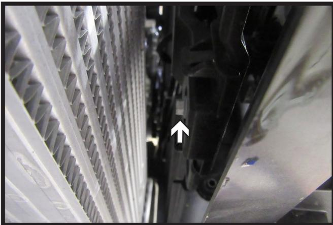
12. Using a 7MM socket, on the backside of the shutters, remove the one (1) bolt from the shutter housing.
