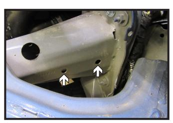
Using a 3/8" drill bit, ream out the two (2) existing holes. Do this on both sides of the vehicle.
