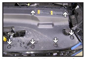
Remove the twelve (12) push pins from the fascia cover. There are six (6) on each side. Set cover aside to be reinstalled later.
