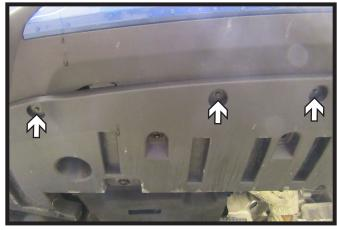
6. Using a 5.5MM socket, remove the ten (10) bolts from the underside of the fascia. There are five (5) on each side.
