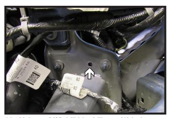
11. Using a 3/8" drill bit, drill one (1) hole as indicated on both sides of the vehicle then install the provided 3/8" hardware.
