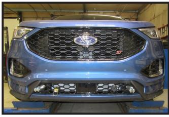
20. Hold the fascia as close to its original position, mark and trim the fascia around the convenience links and attachment tabs. Reinstall the fascia, fascia cover, and headlights.
