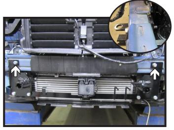
16. Install the 1/2" Bolts with lock washer and a nut plate on the back side. Do this on both sides of the vehicle.
