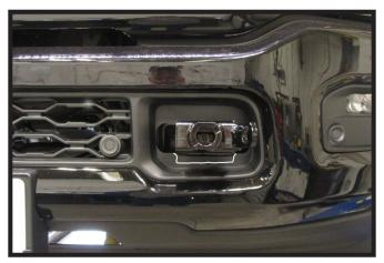
Slide baseplate into tow hook housing as far as possible. Mark plastic for trimming. Do this on both sides of the vehicle.
