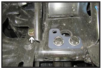
Slide baseplate into place. Insert one (1) 5/8" x 3-1/2" bolt into the existing hole. Do this on both sides of the vehicle.
