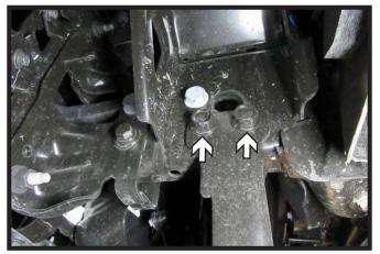
Using a 24MM socket, remove the two (2) bolts from the bracket. Remove bracket, it will not be reinstalled. Do this on both sides of the vehicle.
