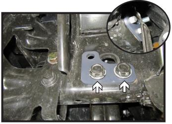
Place spacer brackets on both sides of the frame as shown. Install the two (2) existing 16MM bolts. Do this on both sides of the vehicle.
