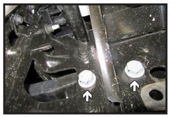
Using a 24MM socket, remove the two (2) bolts from the tow hook. Remove tow hook, it will not be reinstalled. Do this on both sides of the vehicle.
