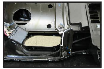
10. Using a reciprocating saw, remove the indicated area on the back side of the fascia to allow room for the baseplate. Do this on both sides of the fascia.
