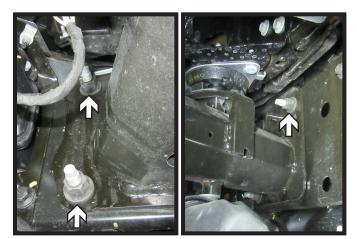
Using an 18MM socket, remove the three (3) bolts from the bumper. Do this on both sides of the vehicle.
