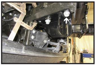
Slide the baseplate onto the frame and start the front 14MM existing bolt. Do not use Loctite<sup>®</sup> Red at this time. Do this on both sides of the vehicle.
