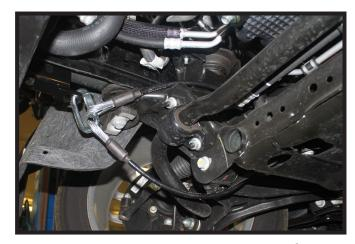
6. Attach the permanent baseplate safety cables to the provided convenience link on the baseplate. The photo shows the recommended installation of the cables to frame of vehicle. Additional options may interfere with suggested mounting; in this case, secure the cables to a solid piece of the frame as described in the General Information sheet. Be sure the safety cables do not rub against any hoses or moving parts. Do this on **BOTH** sides of the vehicle.
