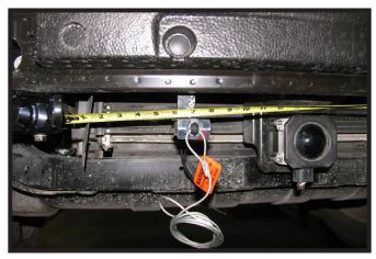
15. **Optional Breakaway:** In the desired location, install the bracket to the bumper with a #10-16 x 1" self drilling screw. Attach the breakaway to the bracket with a 1/4"-20 x 3/4" bolt and 1/4"-20 lock nut.
