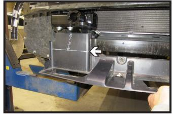
7b. **2021 Models:** Hold the plastic shield up to the push pin holes and trim shield approximately 3" as shown for baseplate clearance.
