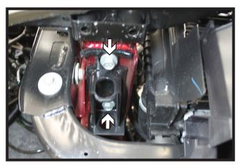
3. **Models equipped with tow hooks:** Using a 16MM socket, remove the two (2) bolts from the tow hook bracket. Remove the tow hook bracket from the vehicle. Do this on both sides of the vehicle.
