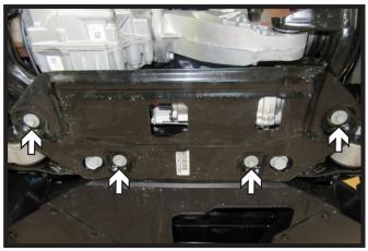
8. Using a 13MM socket, remove the four (4) bolts from the metal belly pan. Remove metal belly pan and set aside to be reinstalled later.
