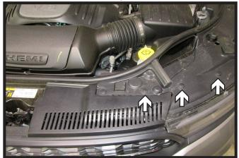
1. Remove the six (6) push pins, three (3) on each side, from the top edge of the fascia.
