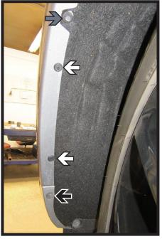
2. In the wheel well, using a 10MM socket, remove the top screw (gray). Using a 8MM socket, remove the lower screw (black). Then remove the two (2) plastic rivets (white). Do this on both sides of the vehicle.
