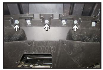
Using a 10MM socket, remove the three
