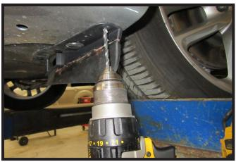
4. Using a 1/4" drill bit, drill out the aluminum pop rivet in front of the tire. Do this on both sides of the vehicle.
