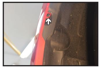
2. Using a 8MM socket or Phillips screwdriver, remove the screw from the top edge of the wheel well. Do this on both sides of the vehicle.
