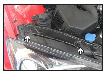
Using a 10MM socket, remove the two (2) screws from the passenger side headlight. Disconnect the wiring and set aside.
