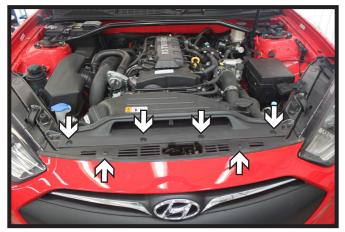
1. Remove the six (6) Phillips head push pins from the top edge of the fascia.
