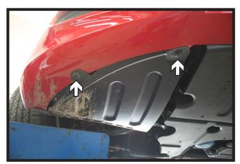
Remove the four (4) Phillips head push pins from the underside of the fascia. There are two (2) on each side.
