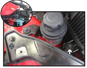
Underneath the passenger side headlight, using a 10MM socket, remove the screw from the brace (white). Then using a 12MM socket, remove the screws from the top and side of the brace (gray).
