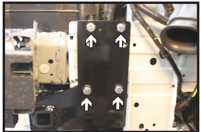
8. Using a 3/8" drill bit, drill the four (4) outer holes in the baseplate thru the frame. Install the 3/8" hardware and fully tighten all bolts. Do this on both sides of the vehicle.
