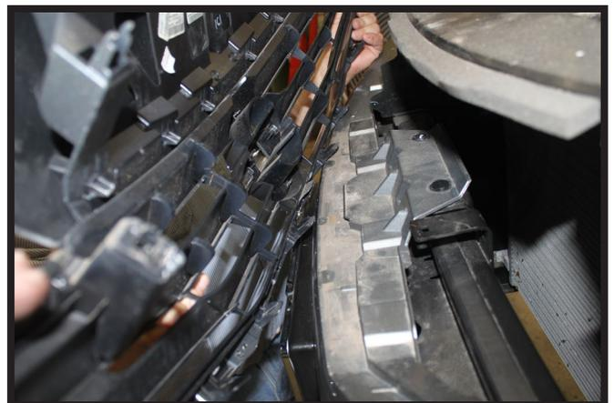
2. Remove the grille from the vehicle by unsnapping the eight (8) clips from along the backside of the grille. Set the grille aside.
