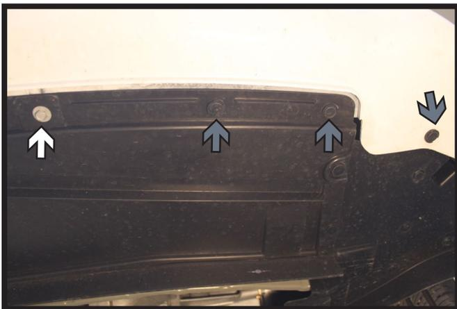
3. Using a 10MM socket, remove the two (2) screws from the under of the fascia. There is one (1) on each side (white).
