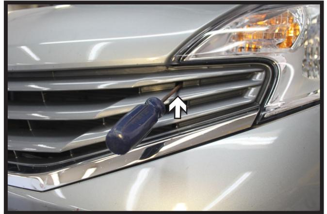
1. Remove the five (5) push pins from the top edge of the fascia. There are two (2) on the driver side and three (3) on the passenger side (left).
