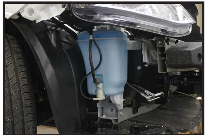
12. Reinstall the washer reservoir on the passenger side.
