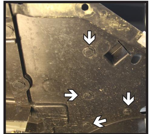
3. Remove the liner from the driver side by removing the one push pin in the wheel well (left). Then the two (2) along side the frame rail (middle) and the four (4) on the underside (right). Set the liner aside it will be reinstalled after baseplate installation.
