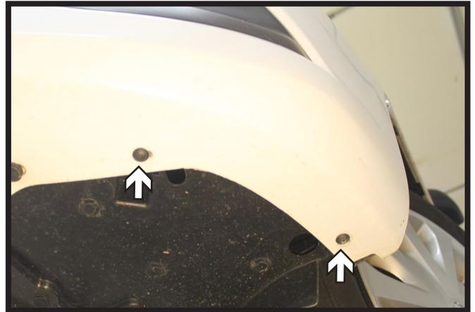
2. Using a T20 Torx, remove the four (4) screws from the underside edge of the fascia. There are two (2) on each side.
