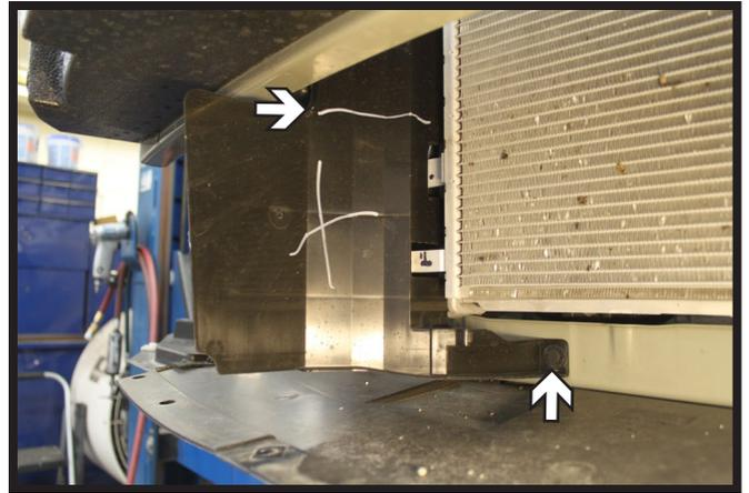
1. Disconnect all lines from the reservoir and plug any fluid lines. Using a 10MM socket, remove the three (3) screws from the washer reservoir.
