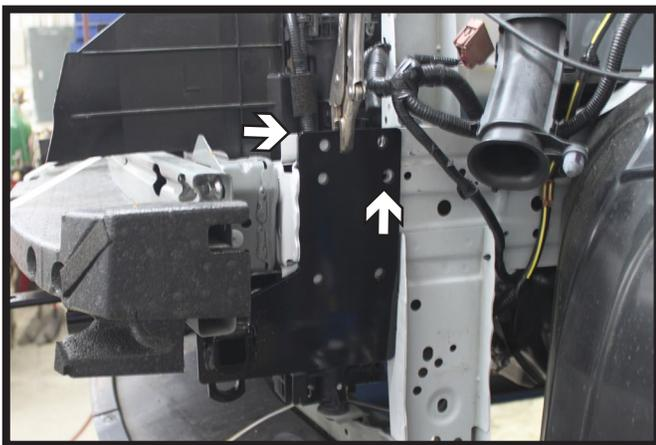
7. Install the baseplate onto the frame, flushing it with the top of the frame rail and centering it on the existing bracket screw hole. Check that the baseplate is level and clamp into place.
