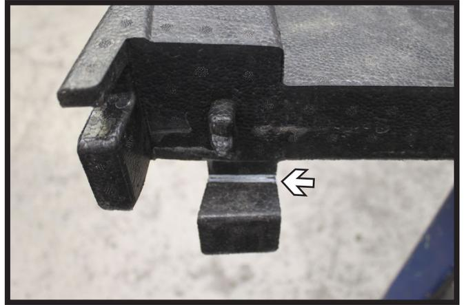
5. **Versa Sedan Only:** On the driver side of the foam reinforcement, trim off the lower tab and reinstall.
