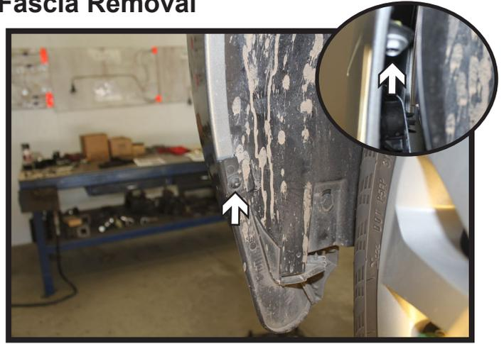
4. Using a T20 Torx, remove the screw from the outer edge of the wheel well. Then using a 10MM socket, remove the screw from behind the wheel well liner. Do this on both sides of the vehicle.
