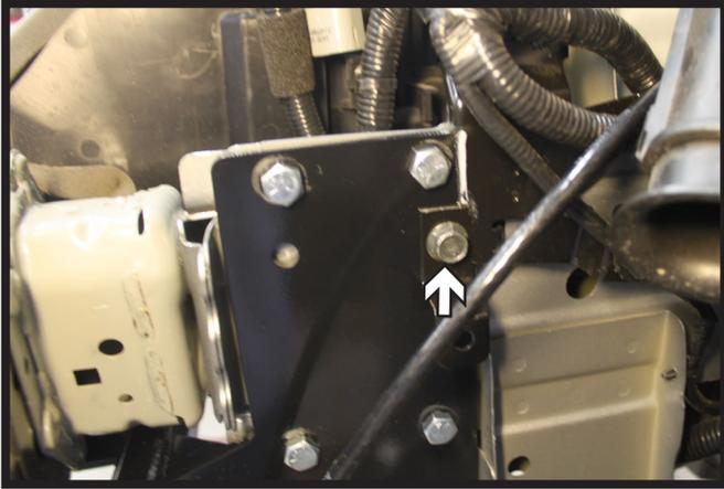
9. Notch the electrical bracket so it will sit vertical and reinstall on the driver side to it's original location with the existing hardware.
