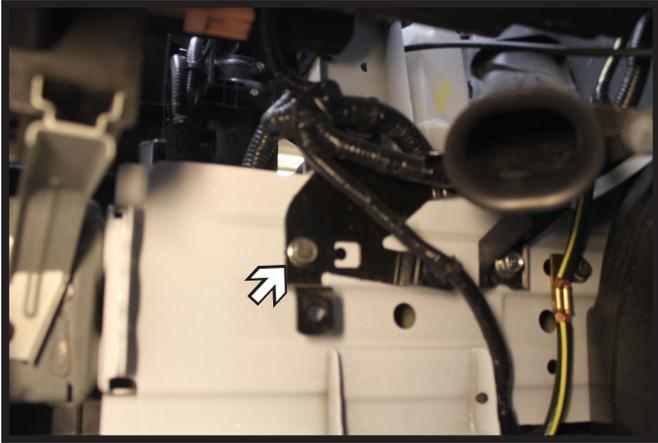
4. On the driver side, using a 13MM socket, remove the screw from electrical bracket and set aside.
