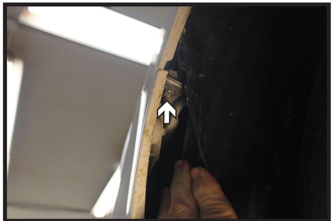
4. Using a 10MM socket, remove the screw from behind the wheel well liner. Do this on both sides of the vehicle.
