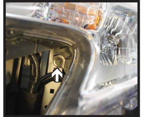
6B. **Versa Note Only:** Using a 10MM socket, remove the three (3) screws from the headlight assembly as shown. Disconnect all electrical connections and set the headlight aside. Do this on both sides of the vehicle.
