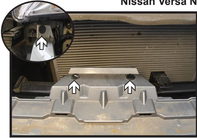
3. Remove the four (4) push pins from the top edge of the fascia. There are two (2) in the middle and one (1) on each side under the headlight.
