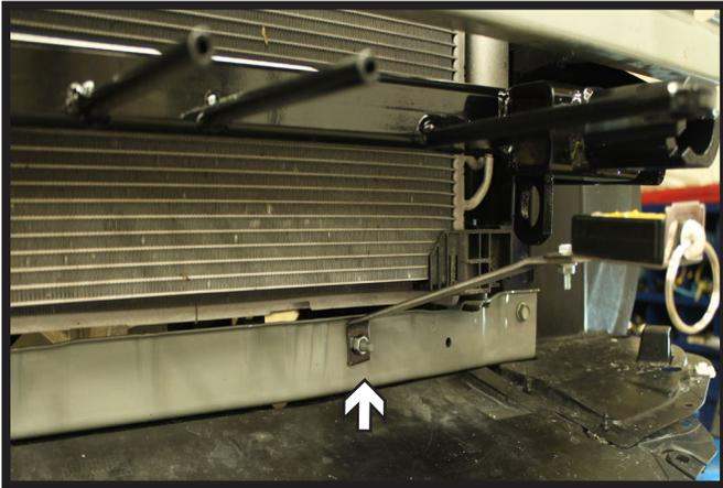
17. **Optional Breakaway:** Attach the bracket to the existing stud and secure with the supplied 8MM hardware. Attach the breakaway to the bracket with the supplied 1/4" hardware.
