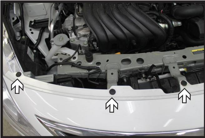
1. Remove the five (5) push pins from the top edge of the fascia. There are two (2) on the driver side and three (3) on the passenger side.
