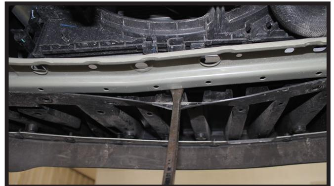
5. Remove the eighteen (18) push pins from the underside of the fascia. There are twelve (12) along the back edge of the belly pan and six (6) along the front edge. Using a T20 Torx, remove the six (6) screws (gray). There are three (3) on each side. Pry the belly pan off the studs, pull the corners of the fascia away from the vehicle disconnecting any electrical connections and set the fascia aside.
