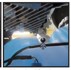
11. Using a 10MM socket, remove the three (3) bolts (white) and one (1) nut (gray) from the windshield washer fluid reservoir on the driver side of the vehicle. Disconnect and plug all lines. Remove reservoir and set aside to be reinstalled later.
