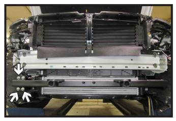
16. Install the remaining three (3) 3/8" bolts with hardware attaching the cross member to the passenger side plate.
