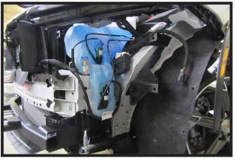
19. Reinstall the windshield washer fluid reservoir on the driver side of the vehicle. Reconnect all lines.
