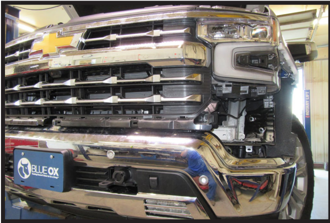
30. Reinstall upper grille piece and reconnect remaining electrical connections.
