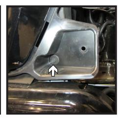
8. Using a 10MM socket, remove the three (3) bolts from the fascia, one (1) in the center and one (1) on each side.
