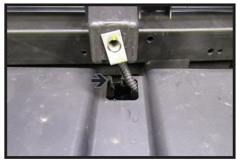
10. Remove seven (7) push pins on the underside of the plastic shroud. Then, either unplug the electrical as indicated (white) or slot the plastic shroud (black) to allow removal. Remove piece and set aside to be reinstalled later.
