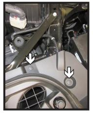
2. Remove the ten (10) push pins from along the top of the fascia. Remove fascia cover and set aside to be reinstalled later.
