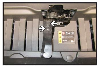
Using a T15 Torx, remove the two (2) bolts from the handle on the top edge of the fascia. Remove and set aside to be reinstalled later.
