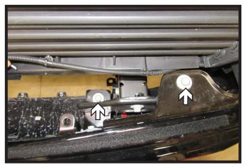
Using an 18MM socket, remove the two
