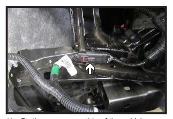
11. On the passenger side of the vehicle unplug the main wiring harness.
