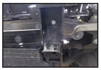
20. Install the 1/2" bolt with hardware into the bottom bolt of the baseplate. Do this on both sides of the vehicle.
