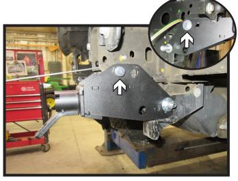
17. Rotate baseplate upward and install the outer front and inner back 1/2" bolts with hardware. Remove the back lower bolt, apply Loctite Red and reinstall. Do this on both sides of the vehicle.
