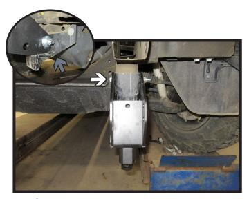
16. Slide baseplate onto tow hook housing so that the back slotted hole of the baseplate lines up with back hole on housing. Insert the one (1) 1/2" x 5" bolt as shown. Leave loose at this time. Do this on both sides of the vehicle.
