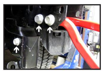
15. Remove the plastic piece from the tow hook. Then using an 18MM socket, remove the three (3) bolts. Do this on both sides of the vehicle. Remove tow hook, it will not be reinstalled later.
