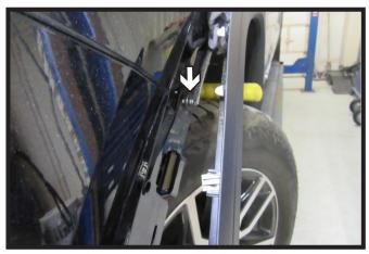
5. Unclip the fender flare and then using a 7MM socket, remove the one (1) bolt. Do this on both sides of the vehicle.
