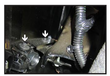
6. Pull back the wheel well liner. Using a 10MM socket, remove the two (2) bolts as indicated. Do this on both sides of the vehicle.
