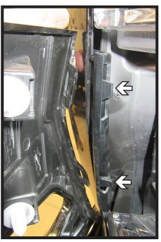
7. Unclip the plastic piece in the center of the headlight by pushing toward the center of the vehicle. Do this on both sides of the vehicle.
