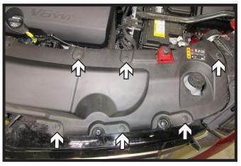
1. Remove the twelve (12) push pins from the fascia cover on the top of the vehicle. There are six (6) push pins on each side of the vehicle. Remove fascia cover and set aside to be reinstalled later.
