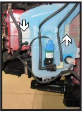
On the driver side of the vehicle, using a 10MM socket, remove the one (1) nut from the top of the windshield washer fluid reservoir. Disconnect all lines. Then using a 10MM socket, remove the two (2) bolts at the bottom of the reservoir. Set aside to be reinstalled later.
