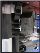
12. Using a reciprocating saw, trim the brackets on the driver and passenger sides of the vehicle as indicated to allow clearance for the baseplate.
