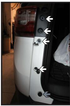
1. Unpop the covers for the five (5) bolts on the back panel of the vehicle. Then using a 7MM socket, remove the four (4) top bolts (white) and use a T20 Torx to remove the one (1) bottom bolt (gray). Do this on both sides of the vehicle.
