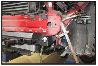
14. Slide baseplate into place. Use large vise grips to hold baseplate in place. Then using a 3/8" drill bit, drill hole in frame using baseplate as a template. Do this on both sides of the vehicle.
