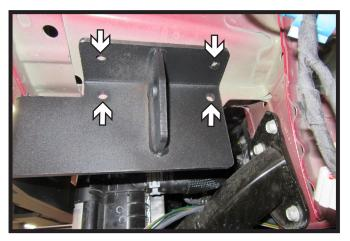
16. Using a 3/8" drill bit, drill the remaining four (4) holes on the side of the vehicle using the baseplate as a template. Do this on both sides of the vehicle.
