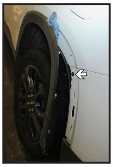
Grab the wheel well trim behind the rear tire and pop out the trim past the side and rear panel joint. Keep trim propped away from panels. Then using a 7MM socket remove the one (1) bolt under the trim. Do this on both sides of the vehicle.
