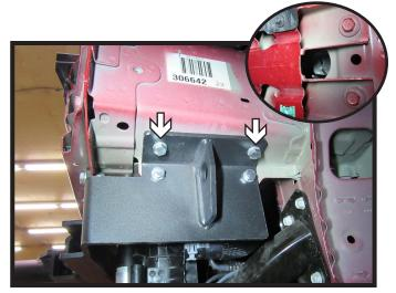
18. Install 3/8" x 1-1/4" bolts with lock washers and nuts plates into top two (2) holes using access hole on front of vehicle (inset). Do this on both sides of the vehicle.
