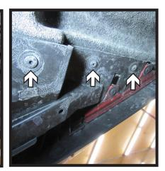
3. Using a T15 Torx, remove the ten (10) bolts from the underside of the fascia. There are three (3) on each side and four (4) in the middle.
