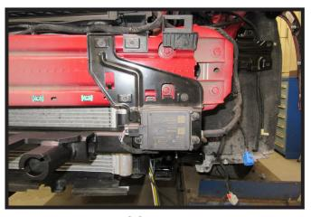
20. Reinstall the ACC bracket on the driver side of the vehicle.
