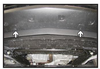
7. Using a T15 Torx, remove the two (2) bolts from the underside of the fascia.
