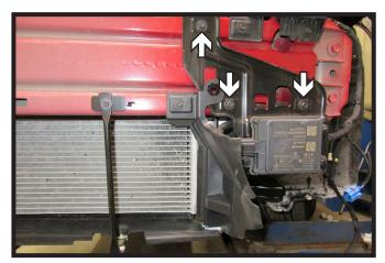
Using a 7MM socket, remove the three
