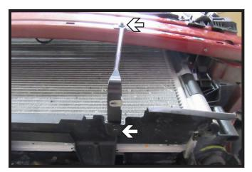
13. Using a 7MM socket, remove the two (2) bolts from the metal bracket on the front of the vehicle. Do this on both sides of the vehicle. These will be reinstalled later.
