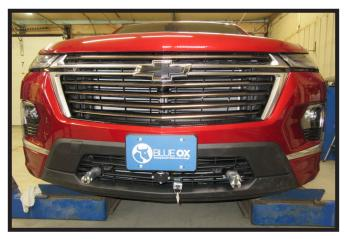
23. Hold the fascia as close to its original position, mark and trim the fascia around the convenience links and attachment tabs. Reinstall the fascia, fascia cover and reconnect all electrical.
