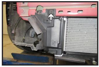
10. Using a 7MM socket, remove the two (2) bolts, one (1) on each side from the top of shroud. Using a utility knife remove the side pieces of the shroud as indicated.
