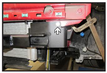
15. Install one (1) 3/8" x 1-1/4" bolt with lock washer and lock nut. Do this on both sides of the vehicle. Remove vise grips.
