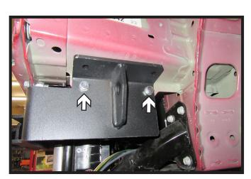
17. Install 3/8" x 1-1/4" bolts with lock washers and lock nuts into bottom two (2) holes. Do this on both sides of the vehicle.
