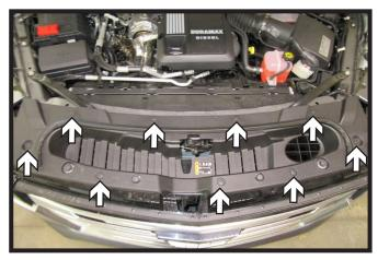
1. Remove the nine (9) push pins from the fascia cover. Remove cover and set aside to be reinstalled later.
