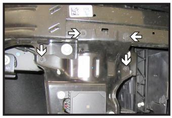
14. **Models with ACC:** Using a 7MM socket, remove the four (4) bolts from the ACC bracket on the passenger side of the vehicle. Set aside to be reinstalled later.
