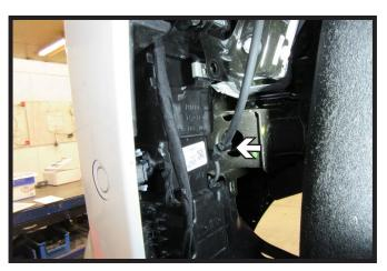
Disconnect washer tube on the driver side of the vehicle. Remove fascia and set aside to be reinstalled later.
