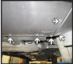
7. Using a 7MM socket, remove the twelve (12) bolts from the side and back of the skid plate.
