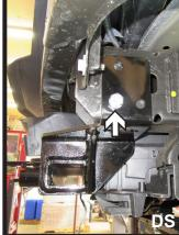
17. Slide the baseplate onto the vehicle and install three (3) 1/2" bolts with lock washers and whiz nuts, two (2) bolts on the passenger side and one (1) on the driver side.
