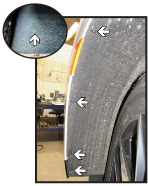
3. Using a T15 Torx, remove the five (5) bolts from the wheel well liner. Do this on both sides of the vehicle.
