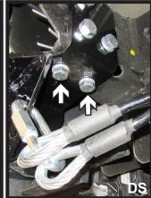
Using a 1/2" drill bit, drill the bottom two
