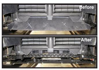
16. Using a reciprocating saw cut along the bottom back edge of the shroud as shown and remove bottom piece.
