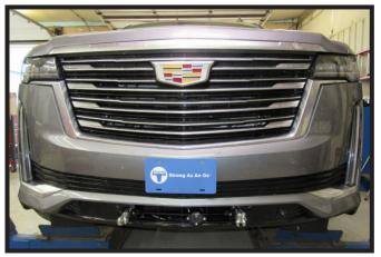
22. Hold the fascia as close to its original position, mark and trim the fascia around the convenience links and attachment tabs. Reinstall the fascia, fascia cover and reconnect all electrical connections.
