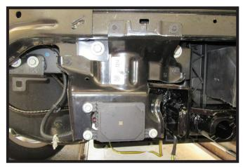
20. **Models with ACC:** Hold ACC bracket up to the vehicle. Mark and trim bracket to allow clearance for the baseplate. Slide the ACC sensor back through hole in bracket and reinstall sensor onto bracket and then bracket onto the vehicle.
