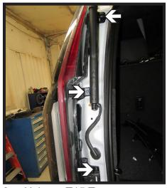
Using a T15 Torx, remove the three (3) bolts attaching the tail light to the vehicle.
