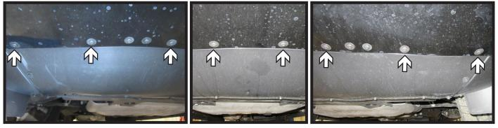
6. Using a T15 Torx, remove the eight (8) bolts from the front edge of the belly pan.
