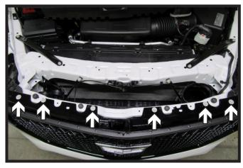
2. Using a 10MM socket, remove the six (6) bolts for the top of the fascia.
