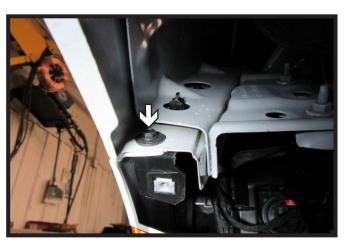
4. Pull back the wheel well liner. Using a 7MM socket, remove the one (1) bolt from the fascia joint. Do this on both sides of the vehicle.
