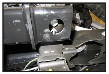
19. Using a 1/2" drill bit, drill the bottom hole on each side of the baseplate. Then install two (2) 1/2" bolts with lock nuts and whiz nuts, one (1) on each side.
