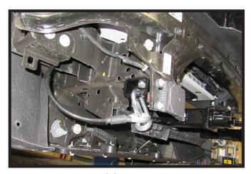
20. Reinstall the ACC bracket on the passenger side of the vehicle.
