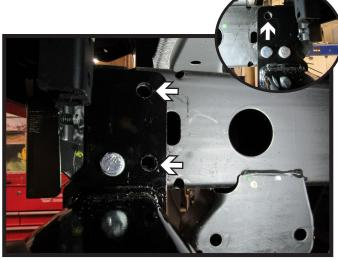
17. Using a 1/2" drill bit, drill the two (2) holes on the passenger side using the baseplate as a template.
