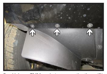
5. Using a 7MM socket, remove the three (3) bolts from the underside of the fascia in front of the tire. Do this on both sides of the vehicle.
