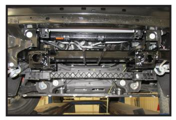
22. Reinstall the belly pan mounting bracket.
