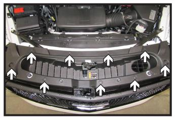
Remove the nine (9) push pins from the fascia cover. Remove cover and set aside to be reinstalled later.
