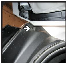
Using a T15 Torx, remove the one (1) bolt at the top of upper plastic cover. Remove upper cover.
