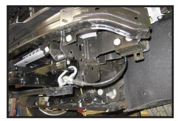
21. Attach the permanent baseplate safety cables to the provided convenience link on the baseplate. The photo above shows the recommended installation of the cables to frame of vehicle. Additional options may interfere with suggested mounting; in this case, secure the cables to a solid piece of the frame as described in the General Information sheet. Be sure the safety cables do not rub against any hoses or moving parts. Do this on **BOTH** sides of the vehicle.
