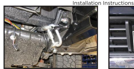
17. Attach the permanent baseplate safety cables to the provided convenience link on the baseplate. The photo above shows the recommended installation of the cables to frame of vehicle. Additional options may interfere with suggested mounting; in this case, secure the cables to a solid piece of the frame as described in the General Information sheet. Be sure the safety cables do not rub against any hoses or moving parts. Do this on **BOTH** sides of the vehicle.
