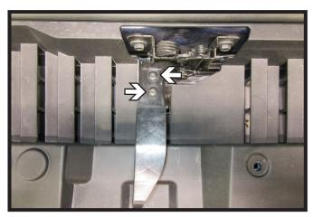
1. Using a T15 Torx, remove the two (2) bolts from the handle. Remove handle and set aside to be reinstalled later.
