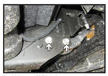
Using an 18MM socket, remove the two
