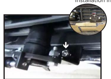
20. Using a 1/4" drill bit, drill two (2) holes on the passenger side of the vehicle using the electrical bracket as a guide. Insert two (2) 1/4" bolts with hardware.
