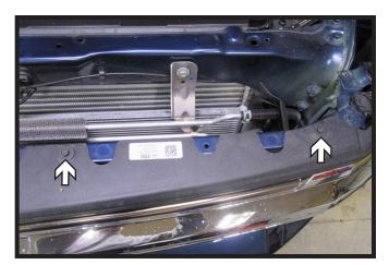
Using a 10MM socket, remove the two (2) bolts from the top of the fascia. Do this on both sides of the vehicle.
