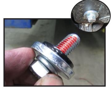
16. Insert one (1) 1/2" bolt with lock washer, thick washer, and slotted washer into the bottom of baseplate. Once bolt is started, position slotted washer and tick washer then tighten bolt. Do this on both sides of the vehicle.
