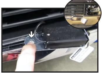
21. Optional: Using a 1/4" drill bit, drill one (1) hole on the driver side of the vehicle. Attach breakaway switch using one (1) 1/4" bolt with hardware. Note: Install where indicated to breakaway cord through opening in fascia and avoid shutters (inset).
