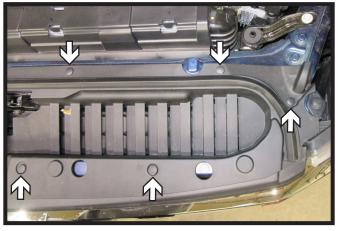
2. Remove the ten (10) push pins from the top of the fascia, there are five (5) on each side. Remove fascia cover and set aside to be reinstalled later.
