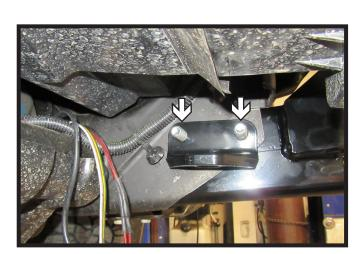
15. Slide the convenience link bracket onto the two (2) 1/2" bolts and place a nylon lock nut on each bolt to secure. Do this on both sides of the vehicle.
