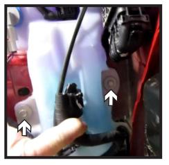
10. Using a 10MM socket, remove the four (4) bolts from the windshield washer fluid reservoir on the driver side of the vehicle. Disconnect all lines. Remove reservoir and set aside to be reinstalled later.
