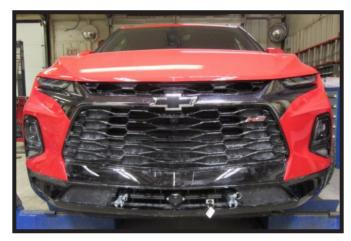
25. Hold the fascia as close to its original position, mark and trim the fascia around the convenience links and attachment tabs. Reinstall the fascia and fascia cover. Reconnect all electrical connections.
