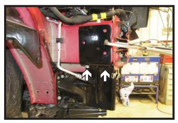
13. Slide the passenger side plate onto the vehicle ensuring that it is as high as possible and as far forward as possible. Using a 3/8" drill bit, drill the two (2) bottom holes and start the two (2) 3/8" bolts with hardware.
