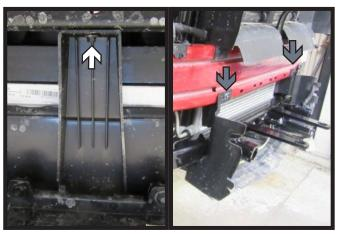
12. Using a 10MM socket, remove the three (3) bolts (white) on the underside of the vehicle holding the plastic shroud. Then using a 7MM socket, remove the two (2) bolts (gray) from above the shroud. Remove shroud and set aside to be reinstalled later.
