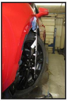
4. Unsnap the fender trim by pulling outward away from the fascia. Place a rag or soft item between the trim and fascia to hold trim out of the way and prevent damage to the fascia. Do this on both sides of the vehicle.
