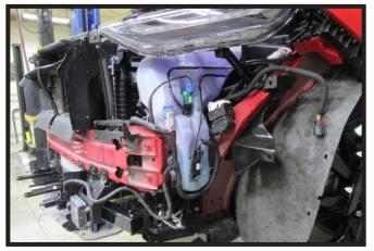
22. Reinstall the windshield washer fluid reservoir on the driver side of the vehicle. Reconnect all lines.
