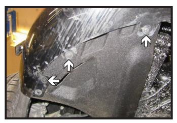
6. Using a T15 Torx, remove the six (6) bolts from the underside of the vehicle in front of the tire. There are three (3) on each side.
