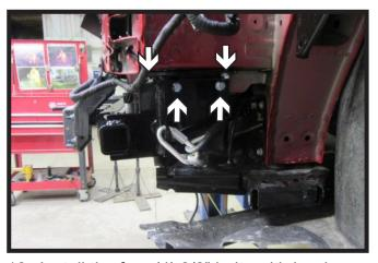
16. Install the four (4) 3/8" bolts with hardware on the driver side of the vehicle.
