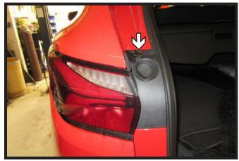
Next to the tail light, pull on the black piece from the top to remove. Do this on both sides of the vehicle.
