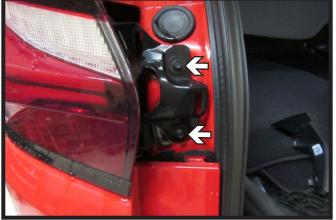
2. Using a 7MM socket, remove the two (2) bolts attaching the tail light to the frame. To remove, push tail light side ways slightly to unsnap and then pull straight back. Do this on both sides of the vehicle.
