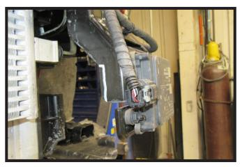
11. On the driver side of the vehicle use a reciprocating saw to trim the back of the Adaptive Cruise Control (ACC) bracket approximately 1/4 inch or more to allow clearance for the baseplate.
