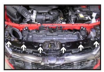
2. Using a T15 Torx, remove the six (6) bolts, three (3) on each side, from the top of the fascia.
