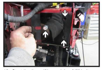
18. Start the three (3) remaining 3/8" bolts with hardware on the passenger side of the vehicle. Insert shim as shown and tighten all hardware. Reinstall the two (2) bumper bolts.
