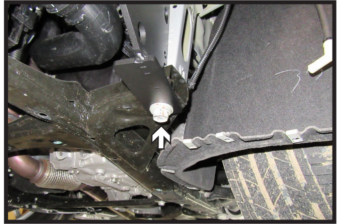
15. Reinstall the existing 14MM bolt into the bottom of the baseplate. Do this on both sides of the vehicle.
