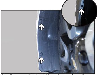
2. Remove the two (2) push pins from the wheel well. Pull back the wheel well cover, and using a 20 Torx, remove the screw at the top of the fascia (inset). Do this on both sides of the vehicle.
