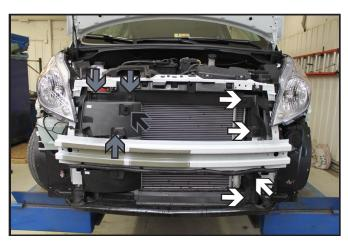
5. Remove the four (4) push pins from the driver side air baffle (white) and set it aside. Then remove the three (3) push pins (gray) and temperature sensor (black) from the passenger side air baffle and remove the baffle from vehicle.
