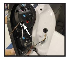
Drill a hole according to the tail light wiring kit instructions.
