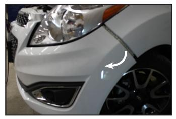
4. Pull the corners of the fascia away from the vehicle disconnecting any electrical connections and set the fascia aside.
