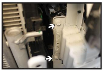
Using a 12MM socket, remove the two (2) bolts from the inside edge of the bumper. Do this on both sides of the vehicle.
