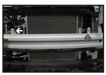
7. Bend the passenger side bumper tab back slightly for baseplate clearance (white).
