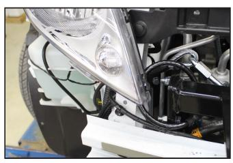
11. Attach the permanent baseplate safety cables to the provided convenience link on the baseplate. The photo shows the recommended installation of the cables to frame of vehicle. Additional options may interfere with suggested mounting; in this case, secure the cables to a solid piece of the frame as described in the instructions included with the permanent baseplate safety cables. Be sure the safety cables do not rub against any hoses or moving parts. Do this on **BOTH** sides of the vehicle.
