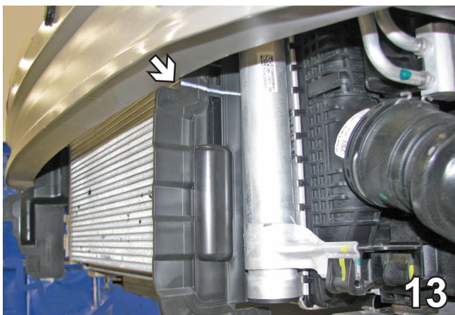
13. Using the utility knife, cut the plastic air dam along the top even with the bottom of the bumper and remove lower section. Do this on both sides.
