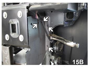
15. Using a 13/32" drill bit, drill the top front hole on each side. Install a 3/8"-16 x 1-1/2" bolt, 3/8" lock washer into the hole and 3/8"-16 nut plate on the inside of the frame (15A). Do this on both sides of the vehicle and fully tighten all fasteners. Drill the remaining holes and install the appropriate hardware(15B). Do this on both sides of the vehicle.
