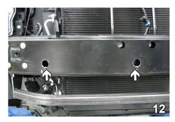
12. Using the 1-1/4" hole saw, drill out the holes in the face of the bumper for the insertion of the nuts. Reattach the coolant line to the back holes using 1/4"-20 x 1/2" hex bolts and 1/4"-20 whiz nuts.
