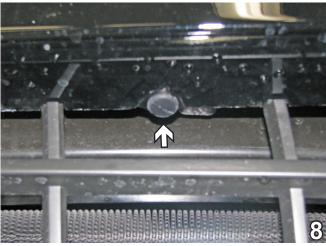
8. **2010-14 Models:** Remove two (2) push pins in the front, one (1) per side.
