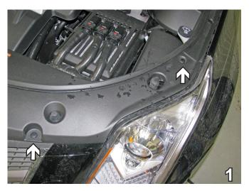
1. Remove the two (2) push pins on each side from the top edge of the fascia. Do this to both sides of the vehicle.
