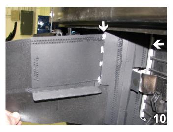
10. Trim the plastic, cut straight down along the seam and straight back under the bumper. Do this on both sides.
