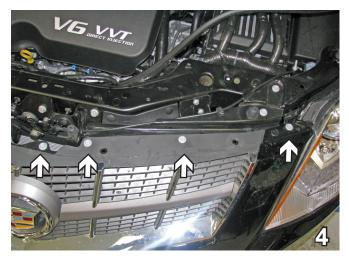
4. Using a 10MM socket, remove seven (7) bolts across the top, three (3) per side and one (1) in the middle.
