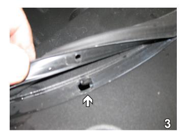
Remove the rubber piece across the top by pulling it to unhook it. Push hard on both sides to release the christmas tree clip.
