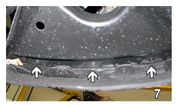
Using a 7MM socket, remove twelve (12) bolts across the bottom of the belly pan.
