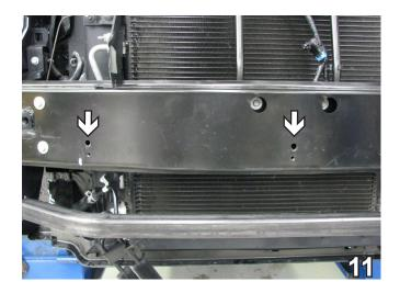
11. Using a 1/4" drill bit, drill into the holes above where the coolant line bolts were taken out. Dril thru the back side of the bumper.
