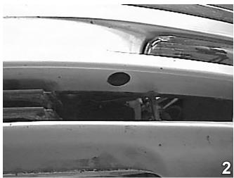
2. Remove the #12 Torx bolts from below the headlight. Do this on both sides of the vehicle. Set bolts aside to be reinstalled later. Unplug the running lights, and pull the fascia forward from the vehicle. Set the fascia carefully aside to be reinstalled later.
