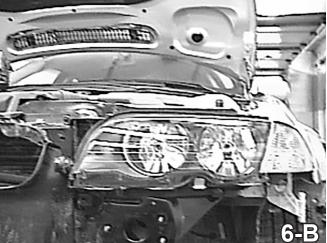
6. Remove the passenger's side headlight only. There are four 8MM bolts, two on the top and two on the bottom that hold it in place. Disconnect the electrical wiring and set headlight assembly and bolts aside to be reinstalled later.
