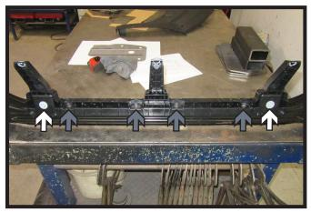
11. Using a 10MM socket, remove the two (2) bolts (white) from the plastic piece on the bottom of the bumper. Then using a 1/4" drill bit, drill out the four (4) plastic rivets (gray). Remove plastic piece and set aside to be reinstalled with the baseplate.
