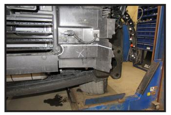
12. Using a utility knife, trim plastic shroud as shown on both sides of the vehicle and remove piece.
