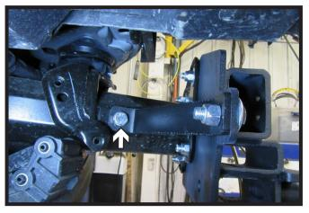
16. Install one (1) 1/2" bolt with lock washer and whiz nut. Do this on both sides of the vehicle.
