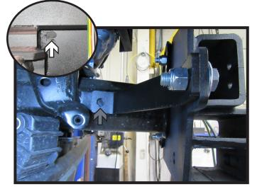
15. Using a 1/2" drill bit, drill the bottom inside hole on the front of the baseplate (inset). Then using the support bracket as a template, drill 1/2" hole in frame (gray). Do this on both sides of the vehicle.
