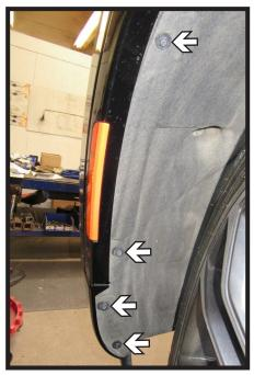
1. Using an 8MM socket, remove the four (4) bolts from the wheel well edge. Do this on both sides of the vehicle.
