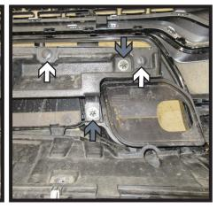
8. Remove the six (6) push pins (white) and five (5) clips (gray) from the foam piece on the back of the fascia. Remove foam piece and set aside, it will not be reinstalled.
