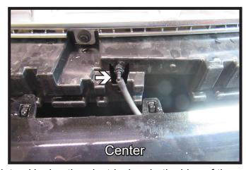
Remove fascia and set aside to be reinstalled later. Unplug the electrical on both sides of the vehicle and hose in the center as the fascia is removed.
