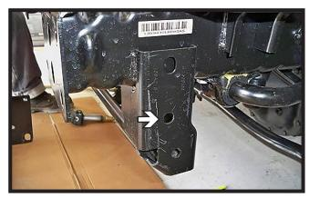
8. On the 2010 models and newer: Align the baseplate's lower hole with the existing middle hole in the frame, ensure baseplate is level with frame and clamp in place with vice grips. Do this to both sides of the vehicle.
