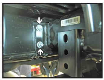
3. Disconnect the foglights from back side of bumper. Using an 18MM socket, remove the two (2) bolts on outside edge of frame. Do this on both sides of the vehicle.
