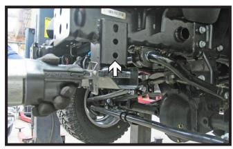
7. On the 2007-09 models: Align the baseplate's lower hole with the existing lower hole in the frame, ensure baseplate is level with frame and clamp in place with vice grips. Do this to both sides of the vehicle.
