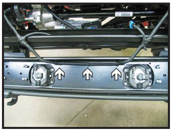
5. Pull the bumper forward and disconnect the three (3) clips attaching the wiring loom along the backside of the bumper. Set the bumper aside to be reinstalled later.
