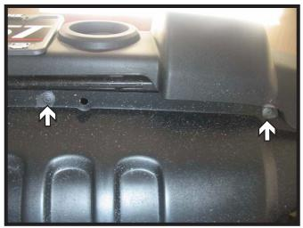
Using a Phillips screwdriver, remove the four (4) push pins from the bottom of the belly pan. There are two (2) on each side.
