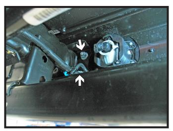
Using an 18MM socket, remove the two (2) bolts on the inside edge of frame. Do this on both sides of the vehicle.
