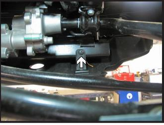
Using a Phillips screwdriver, remove the two (2) push pins from tabs on the backside of the belly pan. Set the belly pan aside to be reinstalled later.
