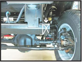
6. On the 2007-09 models: Using the reciprocating saw, cut the lower frame extension flush with the outside edge of the lower side bracket. Do this to both sides of the vehicle. We recommend painting the cut edges to prevent them from rusting.
