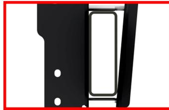
**FIGURE D7:** View showing an incorrectly tightened inside clamp.
