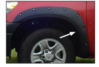
5. Firmly hold flare to fender and mark three locations using holes in flare as a guide. Gently pull back on flare and install three plastic square tabs at marked locations.
