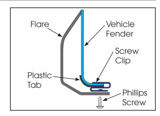
6. Hold flare to vehicle and start factory bolts into existing holes and Phillips screws into holes covered in plastic tabs and clips. *Do not tighten.* Press firmly on flare and tighten all screws. Complete front flare installation.
