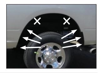
8. Install plastic tab over existing factory hole like Step 5. Install Screw Clip over inner lip edge of fender centered over plastic tab. Install flare using supplied Phillips Screws. Moderate pressure against the flare may be needed for mounting holes to align.
