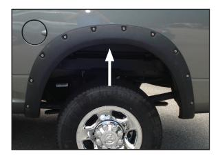
9. Hold flare to vehicle and start supplied Phillips screws and factory bolts into existing holes and holes covered in plastic tabs and clips. *Do not tighten.* Press firmly on flare and tighten all screws. Complete rear flare installation.
