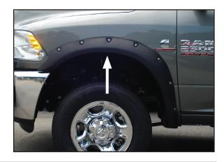
5. Install plastic tab over hole called out in Step 4. Install Screw Clip over inner lip edge of fender centered over plastic tab. Use awl or similar pointed too to put hole in plastic tab through Screw Clip hole. Install flare using supplied Phillips Screws. Moderate pressure against the flare may be needed for mounting holes to align.
