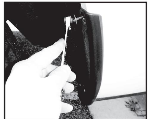
Step 8. Install the rear flare using the factory hardware previously removed. Use one of the supplied phillips head screws in the area indicated by the small arrow. Slight pressure against the outside of the flare pushing towards the vehicle will be needed for installation. Repeat this procedure for the other rear flare.
