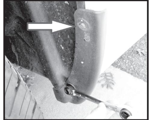
Step 5. Install the flare using the factory hardware previously removed. Use one of the supplied phillips head screws in the area indicated by the small arrow. Slight pressure against the outside of the flare pushing towards the vehicle will be needed for installation. Repeat this procedure for the other front flare.
