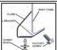
4. Remove the 10 MM bolt in the bottom front area of the rear fender wells. Place the fender flare in place using the 10 MM bolt to position the flare. With a marking pen, mark the mounting holes in the fender well area using the mounting holes in the flare as a guide.
